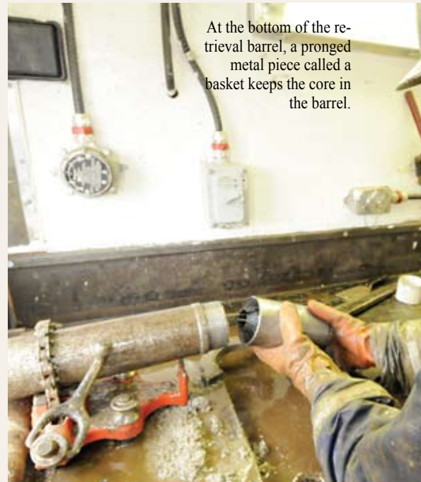
The core retrieval barrel is lowered to the bottom of the hole to extract the core sample.
