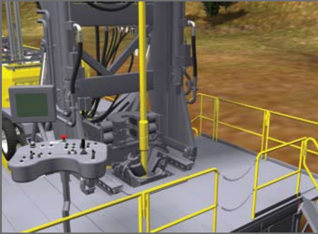
The breakout and pipe handling system is virtually hands free. The console and monitor can be mounted on the work floor or in a control cabin.
