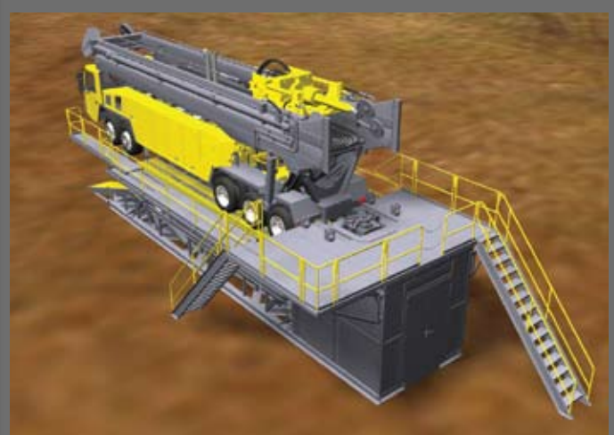
The large work floor is designed to provide ample working space and is configured with crew efficiency and safety in mind.
