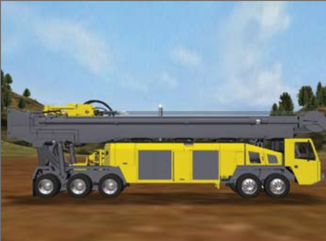
The carrier has a full-width, low-profile cab with the amenities found in conventional trucks. The carrier drive also has the ability to drive in "creep mode," a feature that gives the driver precise control and vehicle placement in off-road or extreme driving conditions.
