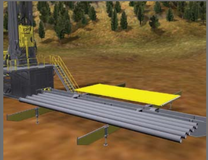
The PREDATOR SKATE is a complete pipe handling system, designed to work with the PREDATOR rig and substructure. It is a single skid-mounted load positioned directly behind the substructure and attached to it. The skate is designed to handle drill pipe, collars and casing. It can handle Range II (30') or Range III (40') oil field drill pipe as well as Range II or Range III lengths of casing up to 24 inches (610 mm) in diameter.
