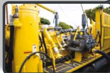
Auxiliary air and booster piping — allows additional air compressor to be hooked up and for air to go through a booster.
