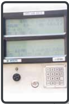
The collected drill data is displayed on this screen and stored.
