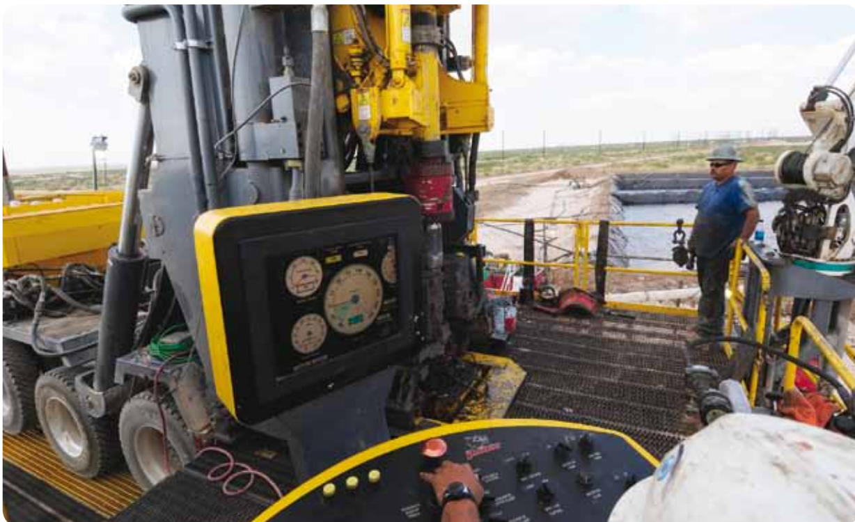
Drill operator Mark Covensky connects the pipe to the rotary head.
