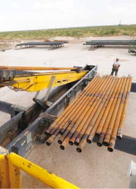
Hector Machuca operates the pipe skate from the ground control box. No hands need touch the pipe except to stab the joint.
