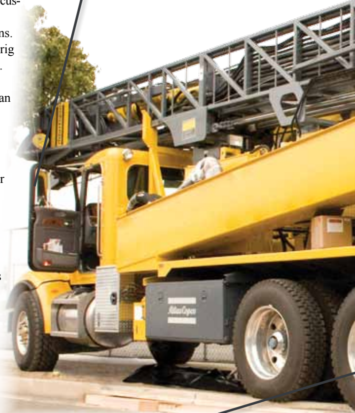
CS14 wireline winch with level wind system to be used for core drilling. Additional PL5 swing in jib winch.
