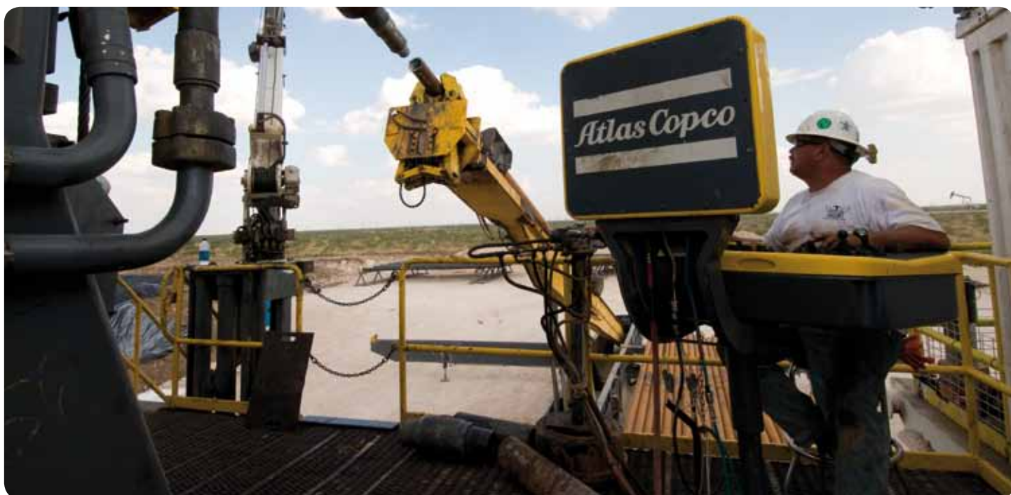
Drill operator Mark Covensky connects the pipe to the rotary head.
