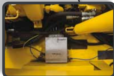
Drill data is collected in a CPU mounted securely on the deck.
