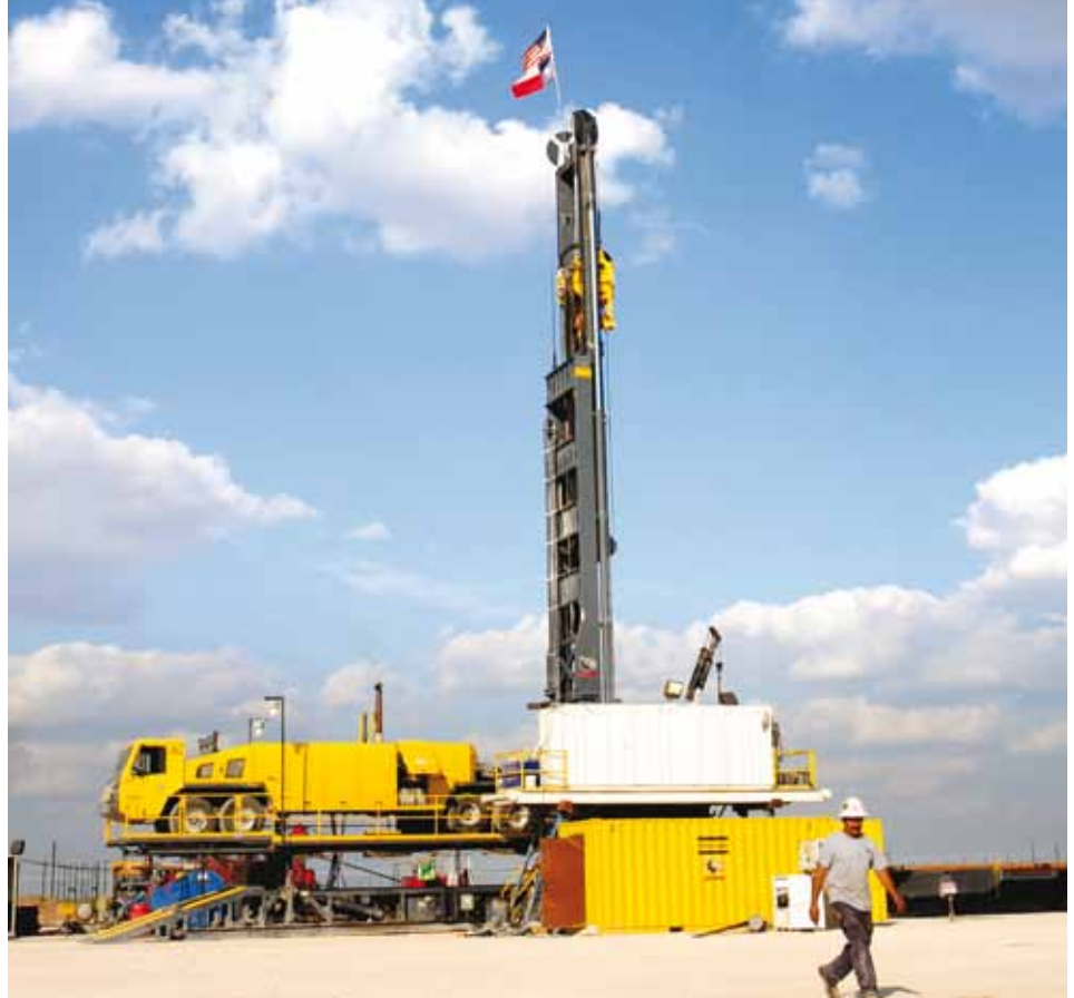
Hector Machuca operates the pipe skate from the ground control box. No hands need touch the pipe except to stab the joint.
