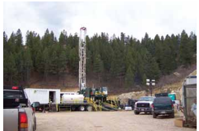
Above: Aerated drilling is underbalanced drilling mixing water, foam and high pressure air.
