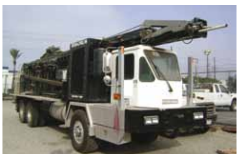
Versa Drill V2000/2003 sn:1120 Location: Milwaukee, WI Tower: 35 ft. 6 in. PTO Engine: CAT C16, 600 hp Drill Hours: 4,443 Compressor: 1,070 cfm / 350 psi
