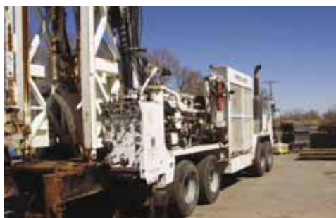
Atlas Copco RD20 III/2001 sn:6660 Location: Denver, CO Tower: 61 ft. Drill Engine: CAT 3412, 735 hp Drill Hours: 13,950 Compressor: 1,250 cfm / 350 psi
