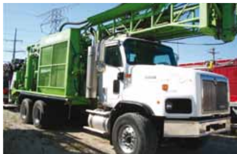
Atlas Copco T3W/2000 sn:6547 Location: Milwaukee, WI Tower: 32' Drill Engine: CAT 15, 565 hp Drill Hours: 6,680 Compressor: 1,070 cfm / 350 psi
