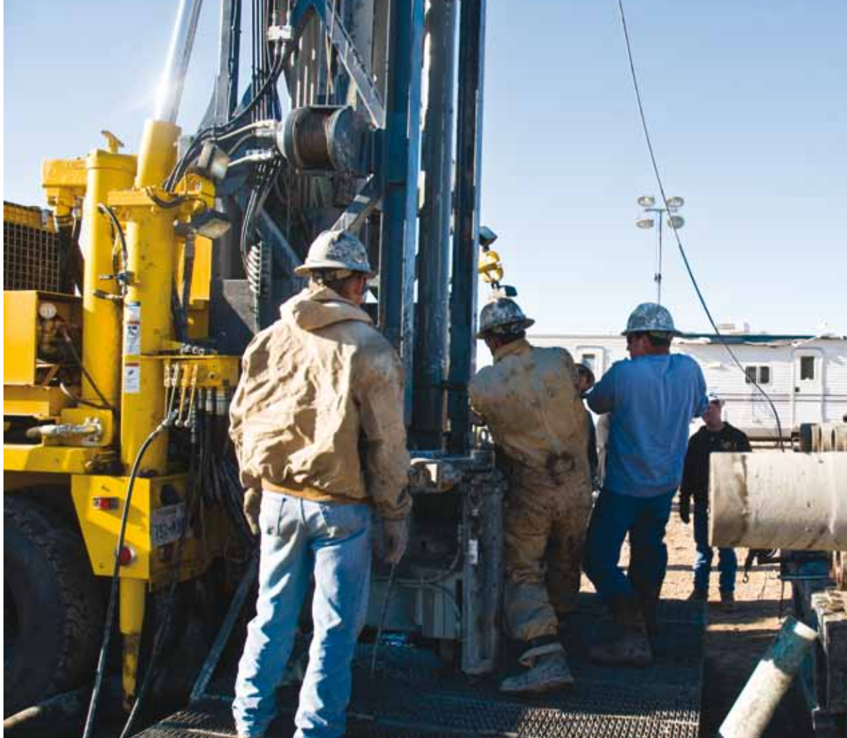
Oil field pipe and collars lack wrench flats, so a chain wrench can be used when the pipe requires manual manipulation.
