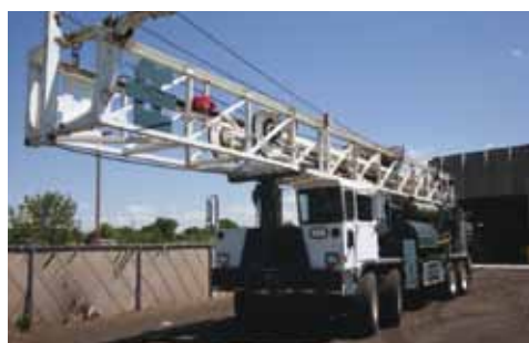
Atlas Copco RD20 III/1998 sn:6389 Location: Denver, CO Tower: 51 ft. Drill Engine: Cummins QSK 19C, 755 hp Drill Hours: 7,972 Compressor: 1,250 cfm / 350 psi
