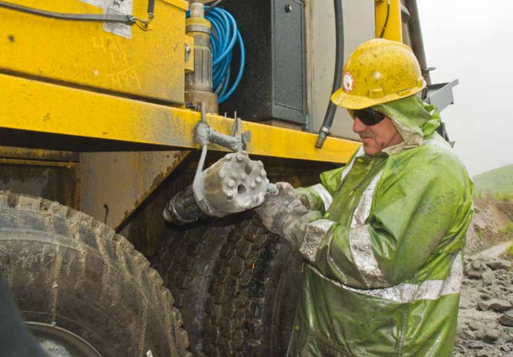
Mike Reinert dresses the carbide buttons on one 6-inch bit to prepare it for its return to drilling.
