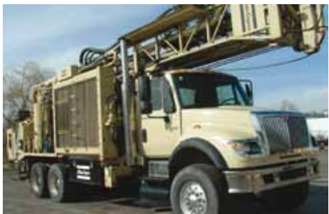
Atlas Copco T3W/2005 sn:6962 Location: Clarks Summit, PA Tower: 32 ft. Drill Engine: CAT C15, 565 hp Drill Hours: 2,157 Compressor: 1,070 cfm / 350 psi
