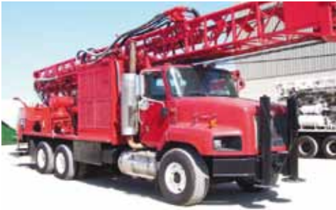
Atlas Copco TH60/2003 sn:6840 Location: Milwaukee, WI Tower: 38 ft. PTO Engine: CAT C15, 565 hp Drill Hours: 7,063 Compressor: 900 cfm / 350 psi
