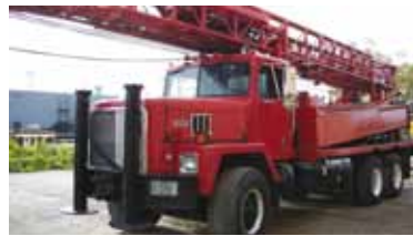
Atlas Copco TH60/1992 sn:3640 Location: Milwaukee, WI Tower: 38 ft. Drill Engine: Cummins N14, 410 hp Drill Hours: 9,207 Compressor: 750 cfm / 300 psi
