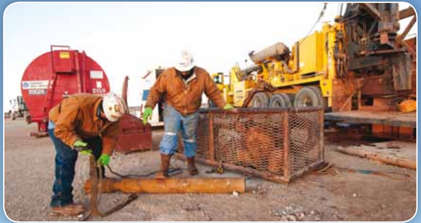
Packing up gear and tooling is quick with the cage and winch. The cage easily loads on a flatbed to move to the next site.
