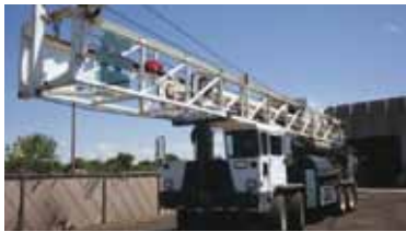
Atlas Copco RD20 II/1998 sn:6389 Location: Denver, CO Tower: 51 ft. Drill Engine: Cummins QSK 19C, 755 hp Drill Hours: 7,972 Compressor: 1,250 cfm / 350 psi
