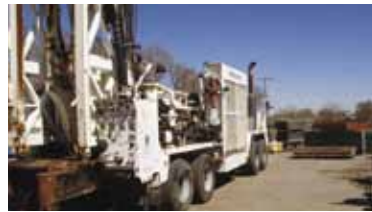
Atlas Copco RD20 III/2001 sn:6660 Location: Denver, CO Tower: 61 ft. Drill Engine: CAT 3412, 735 hp Drill Hours: 13,950 Compressor: 1,250 cfm / 350 psi
