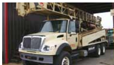
Atlas Copco T3W/2002 sn:6753 Location: Milwaukee, WI Tower: 32 ft. Drill Engine: CAT C15, 565 hp Drill Hours: 6,562 Compressor: 900 cfm / 350 psi
