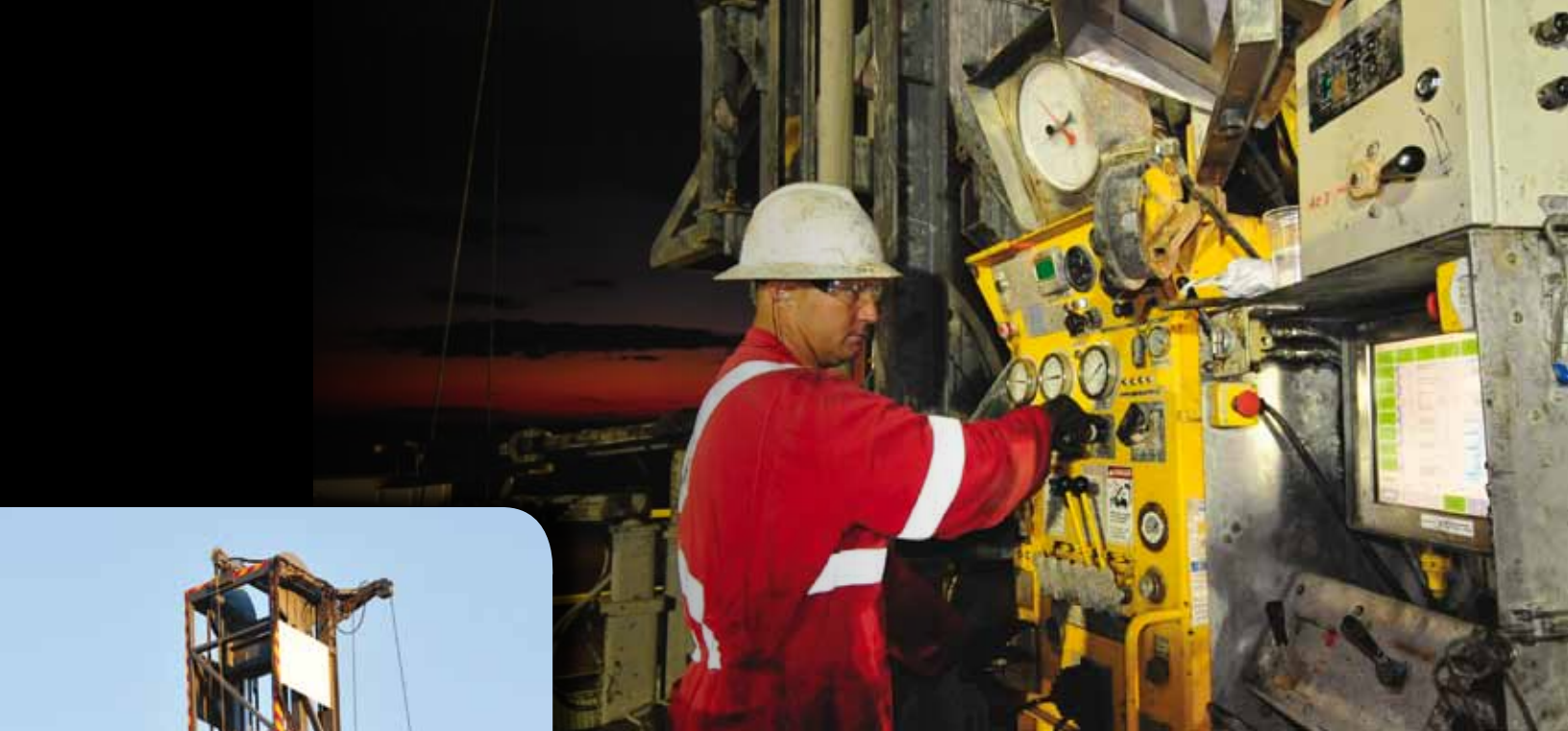
(above) From his position, the driller can see the Pason screen and camera at the top of the tower. The assistant driller operated the pipe handler from a remote control just off his shoulder.
