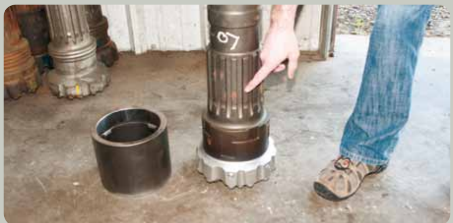
Inside the retrieval sleeve at left can be seen two of the four locking lugs that will engage the grooves below the splines of this bit. The bit and its sleeve, which are sold together as a package, offer drillers and their companies a stress-relieving insurance policy against shanked bits. The sleeve, which attaches to the drill string, catches a broken bit so that it does not have to be fished out nor drilled around.
