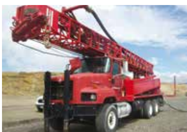
Atlas Copco TH60/2003 sn:6840 Location: Milwaukee, WI Tower: 38 ft. Drill Engine: CAT C15, 525 hp Drill Hours: 7,288 Compressor: 900 cfm / 350 psi
