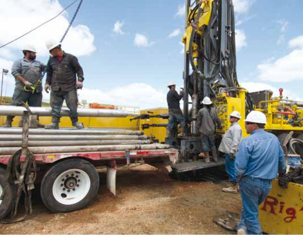
(right) Although the Atlas Copco RD20 can drill to 5,500 ft (1,675 m), it is setting up shallower holes for a conventional oil rig in the Bakken.
