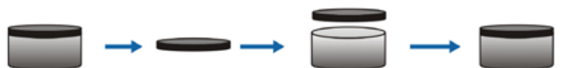
MegaDiamond builds a standard cutter, then removes the diamond table from the substrate. The substrate is discarded and cobalt is removed from the diamond table. The diamond table is then attached to a new substrate. The resulting PDC cutter is deep leached, removing infiltrated cobalt to several hundred microns.
