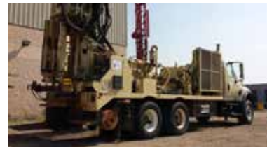
Atlas Copco T2W/2006 sn:6982 Location: Milwaukee, WI Tower: 30,000 lb pulldown/pullback Compressor: 750 cfm/ 300 psi Truck Engine: 525 hp Cat C13 Mud Pump: 3x4 Mission
