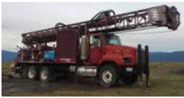
Ingersoll-Rand TH60/2004 sn:6820 Location: Sacramento, CA Tower: 38 ft w/ 29,500 lb pullback Compressor: 900 cfm / 350 psi Truck: International Paystar Truck Engine: 525 hp Cat C15 Mud Pump: 3 x 4 Mission
