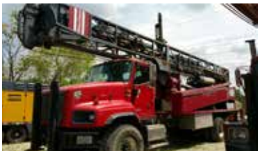
Atlas Copco T3W/2008 sn:21254 Location: Milwaukee, WI Tower: 36 ft w/ 40,000 lb pullback Compressor: 900 cfm / 350 psi Deck Engine: 580 hp Cat C15 Truck: International Paystar Truck Engine: 380 hp Cat C13 Drill Hours: 6,850
