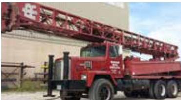
Ingersoll-Rand TH60/1993 sn:3797 Location: Milwaukee, WI Tower: 38 ft. w/ 29,500 lb pullback Compressor: 750 cfm / 250 psi Truck: International Paystar Truck Engine: 410 hp Cummins
