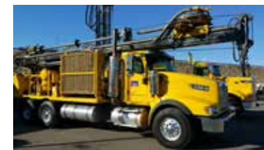
Atlas Copco T2W/2014 sn:21414 Location: Sacramento, CA Tower: 30,000 lb pulldown/pullback Compressor: 900 cfm / 350 psi Truck: International 7600 Truck Engine: Maxforce Drill Hours: 3,000
