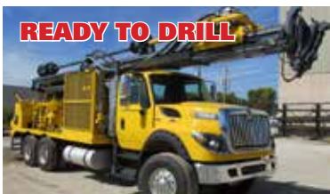
Atlas Copco T2W/2012 sn:21402 Location: Milwaukee, WI Compressor: 750 cfm / 300 psi Tower: 30,000 lb pulldown/pullback Truck: International 7600 Truck Engine: 475 hp IH Maxxforce Drill Hours: 607 Mud Pump: hydraulics in place
