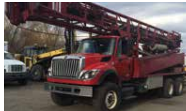
Atlas Copco T3W/2007 sn:21229 Location: Clarks Summit, PA Tower: 36 ft w/40,000 lb pullback Compressor: 900 cfm/ 350 psi Deck Engine: 475 hp Cat C15 Truck: International 7600 Truck Engine: 380 hp C13 Drill Hours: 4239
