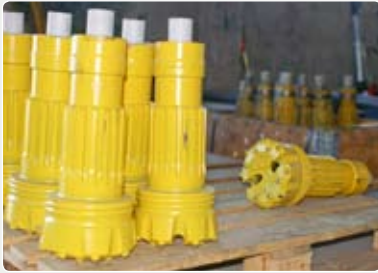
In the bit grinding workshop: New Secoroc button bits and worn bits in the background waiting for regrinding with the Secoroc GrindMatic grinding machine.
