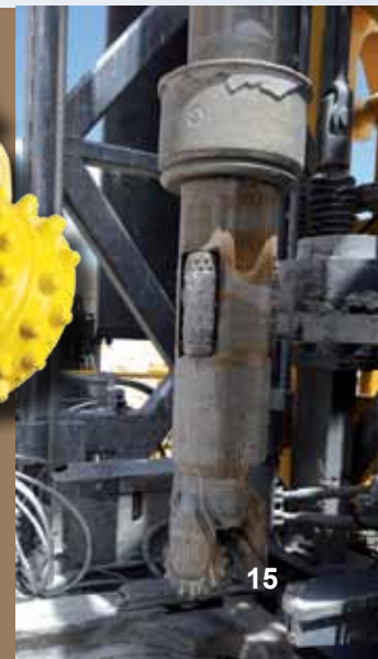
An Atlas Copco Secoroc bit with hole reamer prepares to drill.
