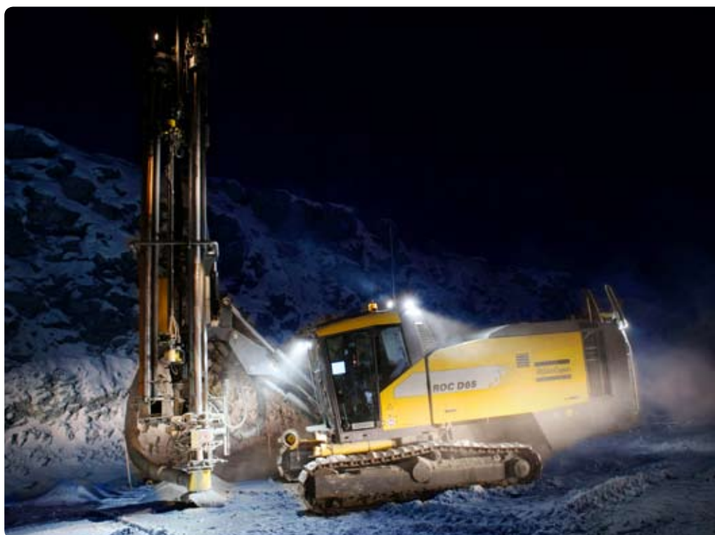
New kid on the block: The SmartRig ROC D65 brings full computerization to DTH drilling in mining thanks to its Rig Control System which automatically controls the drilling cycle.
