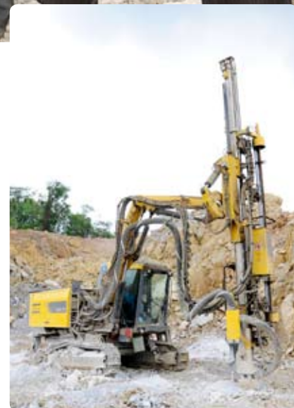
Tackling the boulders: The ROC D7's folding boom system makes it ideal for secondary blasting as well as production drilling.
