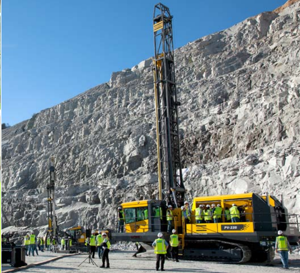
Major attraction: The latest Pit Viper 235 for the hole diameter range 6-0" features the RCS control system and is available in several engine and compressor alternatives for either rotary or high pressure DTH drilling.
