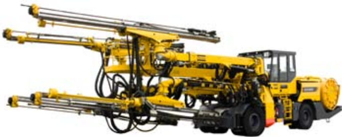
Big boy for a big job: Veidekke's new Boomer XE4 is being used to drive a twin-track tunnel near Gothenburg for high speed trains.
