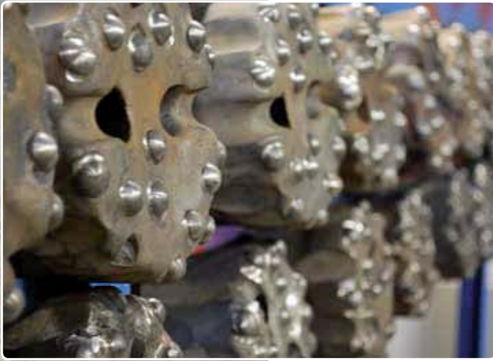
Secoroc bits after grinding: These Secoroc GrindMatic grinding machines make bit grinding easy and efficient in the Aitik workshop.
