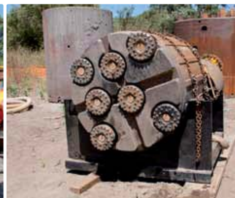
Thor's configuration: A cluster of seven Atlas Copco Secoroc CDS 8-inch hammers equipped with 10-inch bits.
