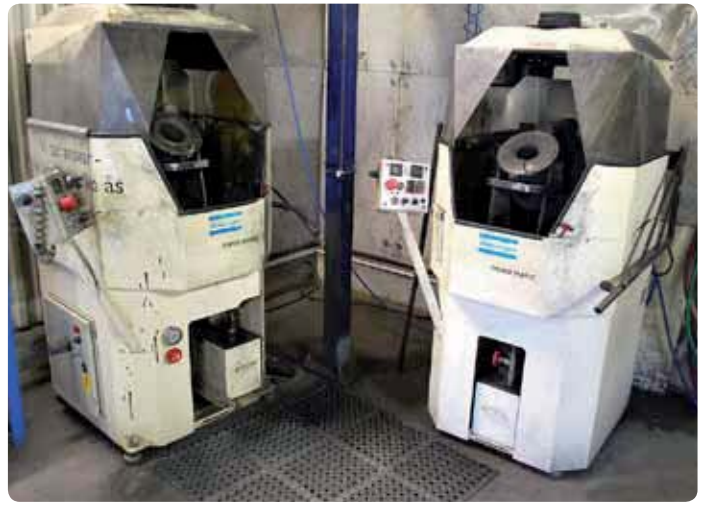
Secoroc bits after grinding: These Secoroc GrindMatic grinding machines make bit grinding easy and efficient in the Aitik workshop.
