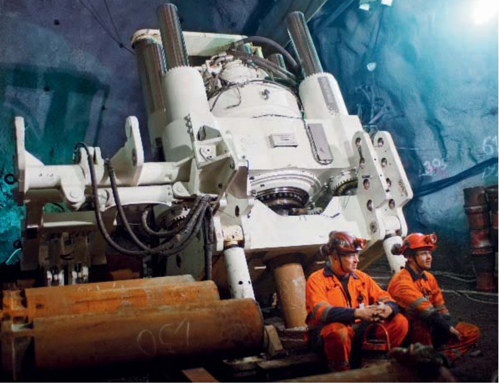
The Atlas Copco Robbins 91RH C raiseborer at Kiruna Mine: A highly advanced machine providing extreme power and torque, pictured here with operators Ulf Lindström and Johan Garp of Bergteam
