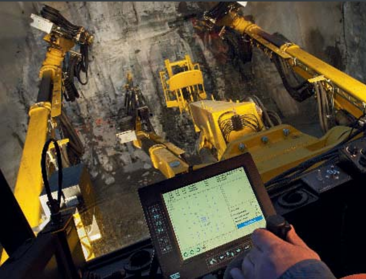
In total control: RCS technology displays all the necessary data on a screen and allows it to be shared with others for total optimization of the operation.
