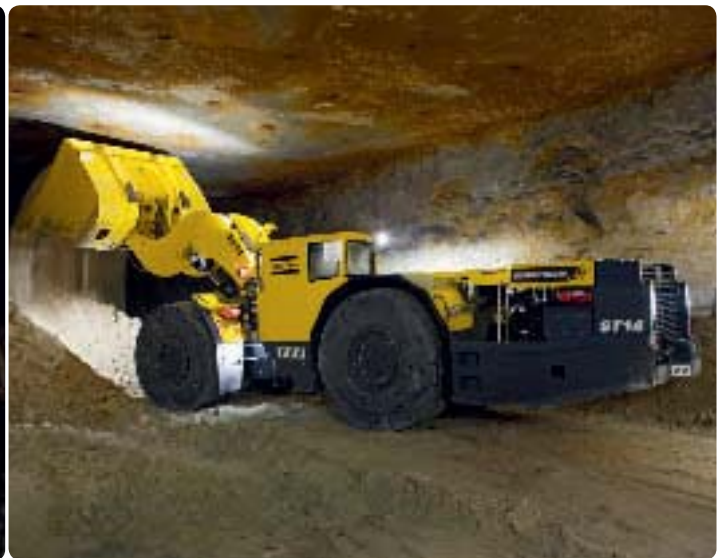
Technology in action: Thanks to the RCS control system, this Scooptram ST14 loader is able to collect and share information on, for example, load weighing, tonnage, and service.
