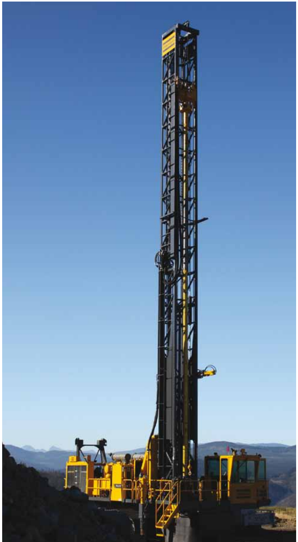
Rapid drilling on the 15-meter benches is easily achieved by 10 5/8-inch Epsilon rotary bits and well matched 2,000-psi air compressor packages, allowing efficient clearing of the holes and increased tool life.
