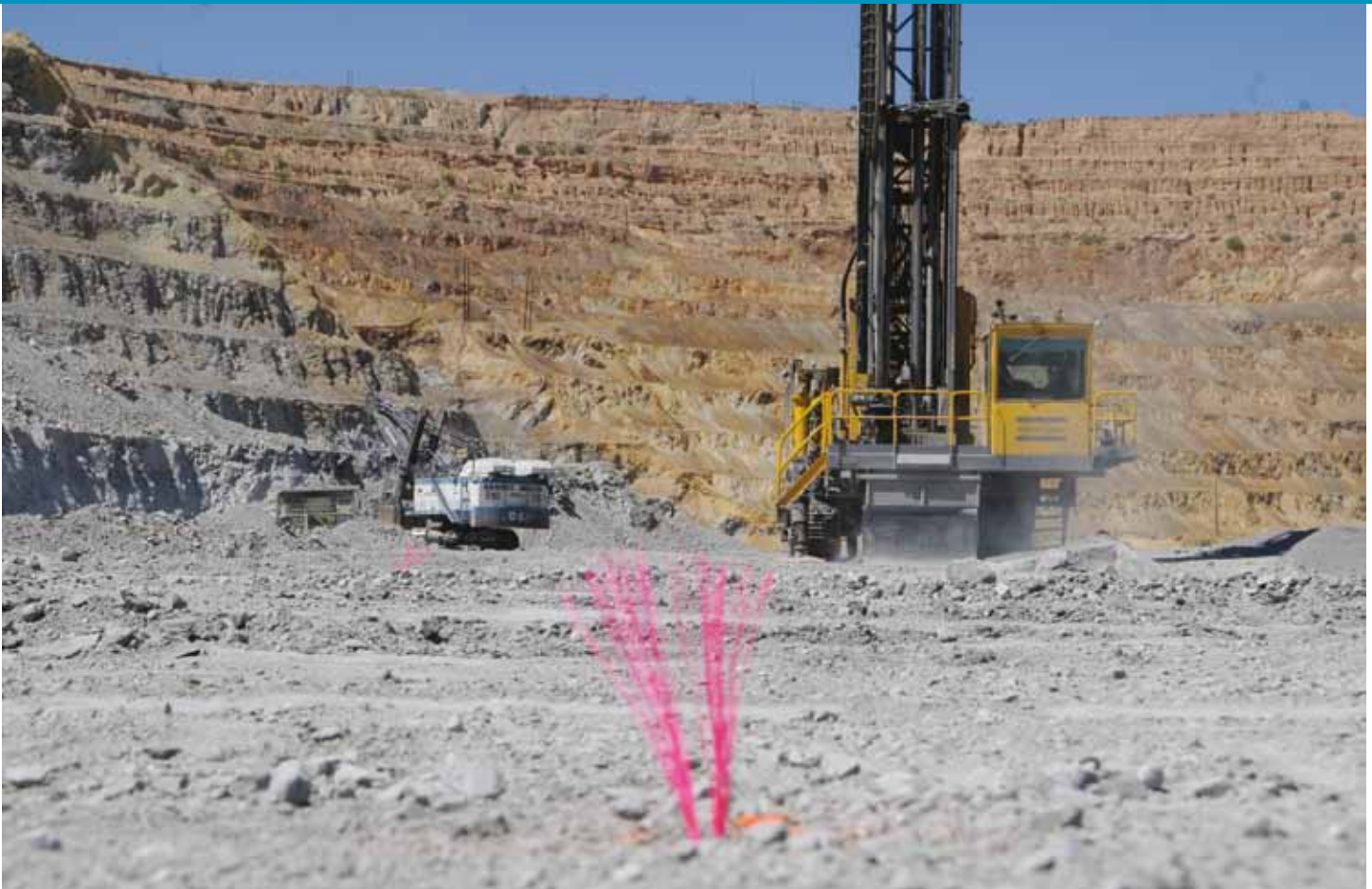
The Diesel Powered PV-271 moves with ease back and forth on the bench increasing productivity by reducing setup time.
