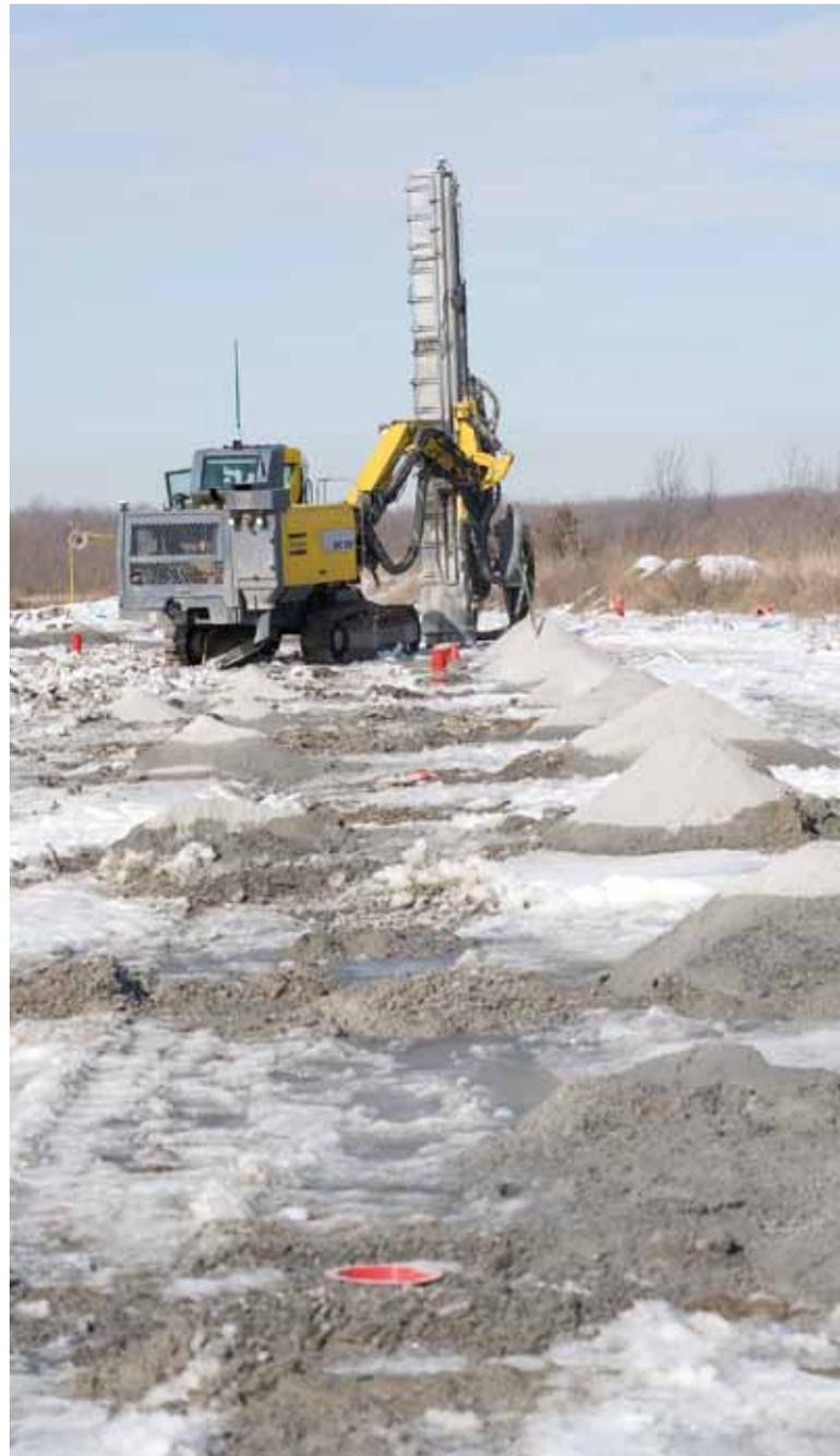
The perfect 4.5 x 5 meter pattern is drilled without physically marking the ground. Bench depth begins at 17 meters at one end with the elevation falling about a foot halfway through the pattern.
