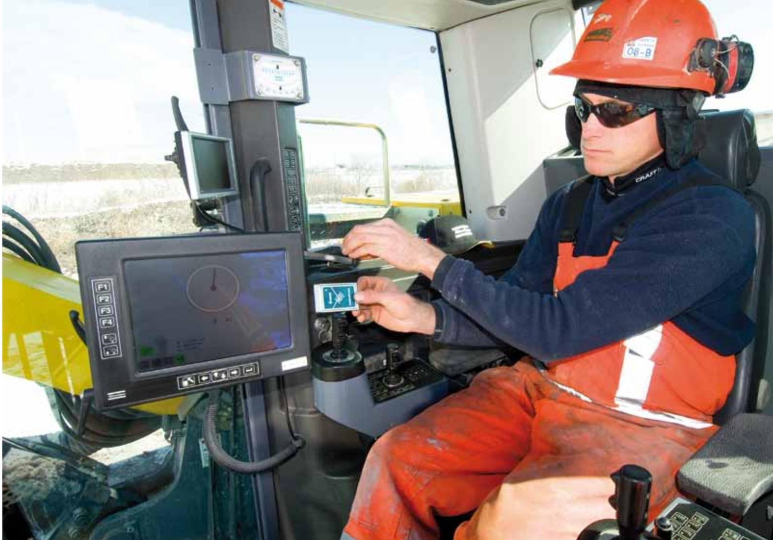
Drill operator John Newton inserts the memory card into the onboard computer. The line in the circle indicates the angle of the feed to the ground. The feed is perfectly straight when the line becomes a dot in the center of the circle.
