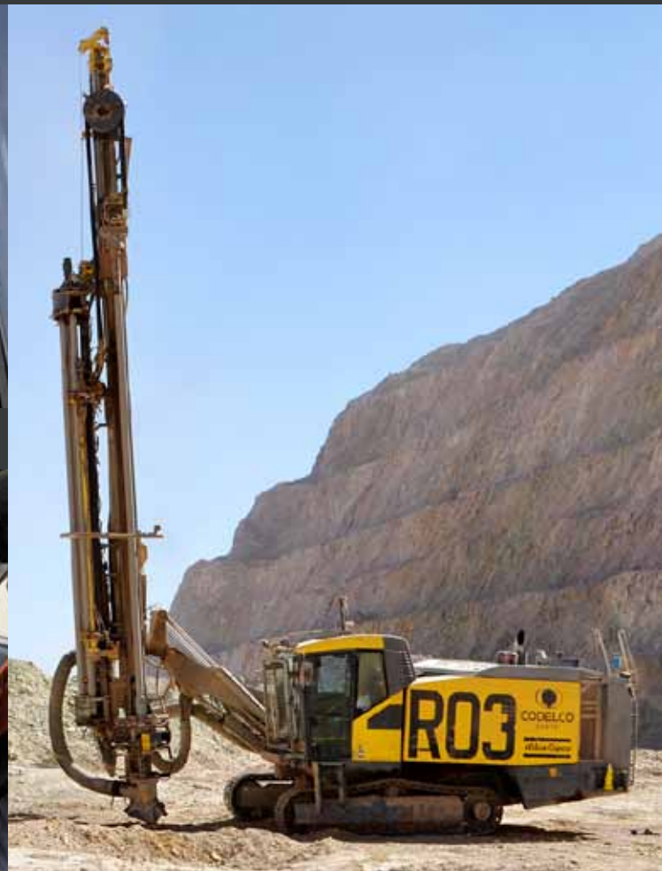
The ROC L8 gets a workout at the mine performing both presplit and production drilling.
