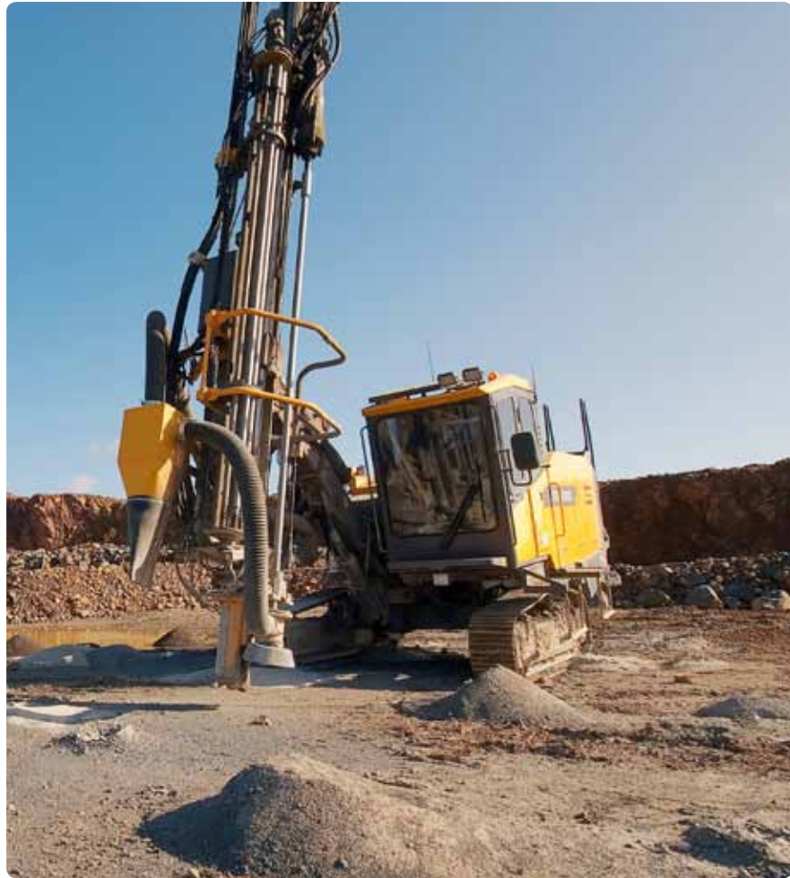
Consistency and reliability: Both PowerROCT35 rigs average 300 m per day for DBS in two separate Queensland quarry sites.
