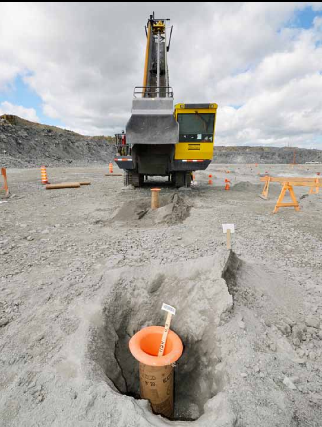
At Malartic, the Pit Viper 235 drills 216 mm (8.5") vertical holes.
