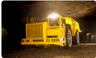
An Australian success story: The 60-tonne Atlas Copco Minetruck MT6020.
