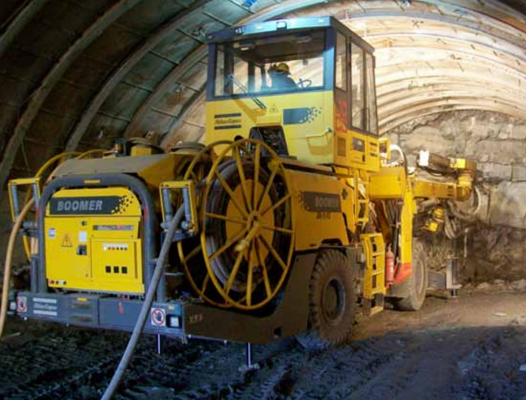
Modern technology for a difficult task: The first Atlas Copco Boomer XE3 C rig in Argentina with the Atlas Copco Rig Control System (RCS) drilling blast holes in the mountains of northwestern Argentina.
