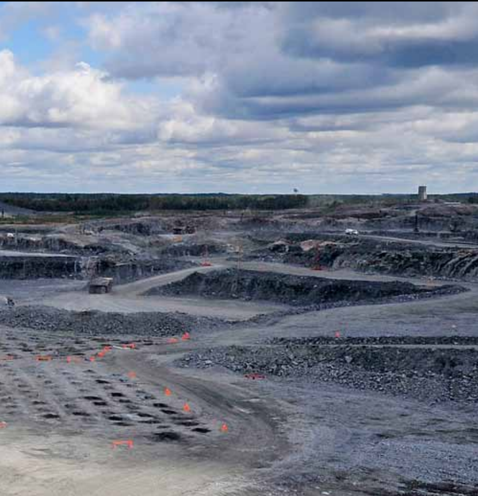
The Pit Viper 235 is used for single pass drilling of 12 m deep holes for the 10 m high benches.
