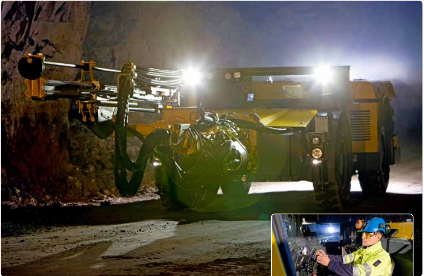
Low and robust: The new Boomer M1 L is specially designed for room and pillar mines with roof heights of 2.2 – 2.5 m. Strength and ease of service are two clear plus points.
