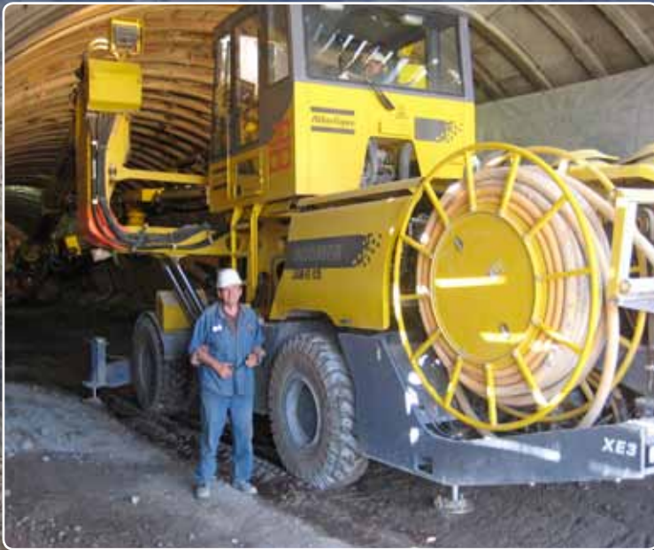
Modern technology rules where the dinosaurs roamed: Far left, the Boomer E2 C carrying out rock support work in the especially difficult Tunnel 3. Left, Fausto Cervini , Tunnel Production Manager with the three-boom Boomer XE3 C in Tunnel 1.
