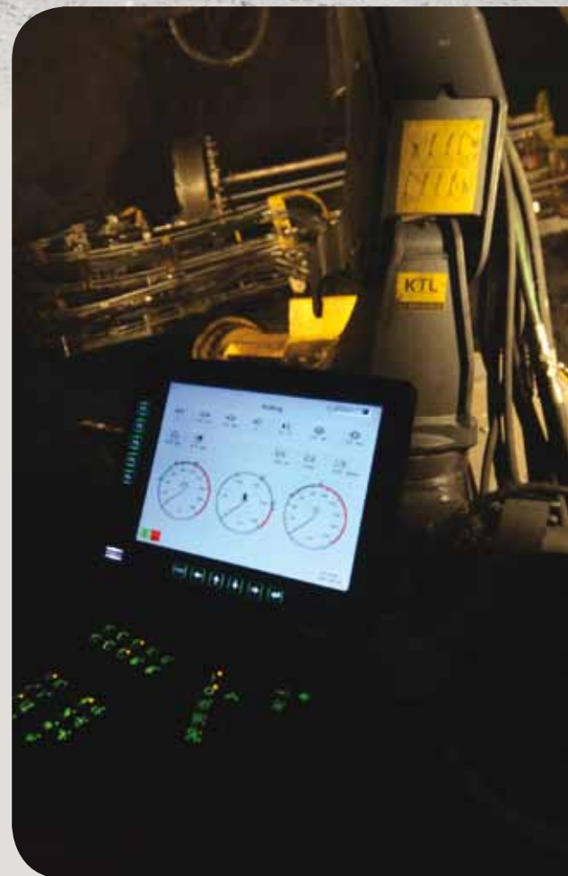
The Boltec's operator monitors performance data from a full-color display above the control console.
