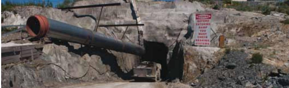
*Although Bell Creek could accommodate 50-tonne mine trucks, the MT42 is the perfect size for their narrow vein operation. With their shorter turning radius and 8 kph speed up the ramps, the three MT42s can haul up to 1,800 tonnes of ore and waste per day.*
