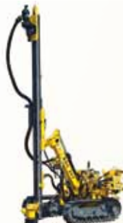
Surface Drilling Equipment (SDE)
