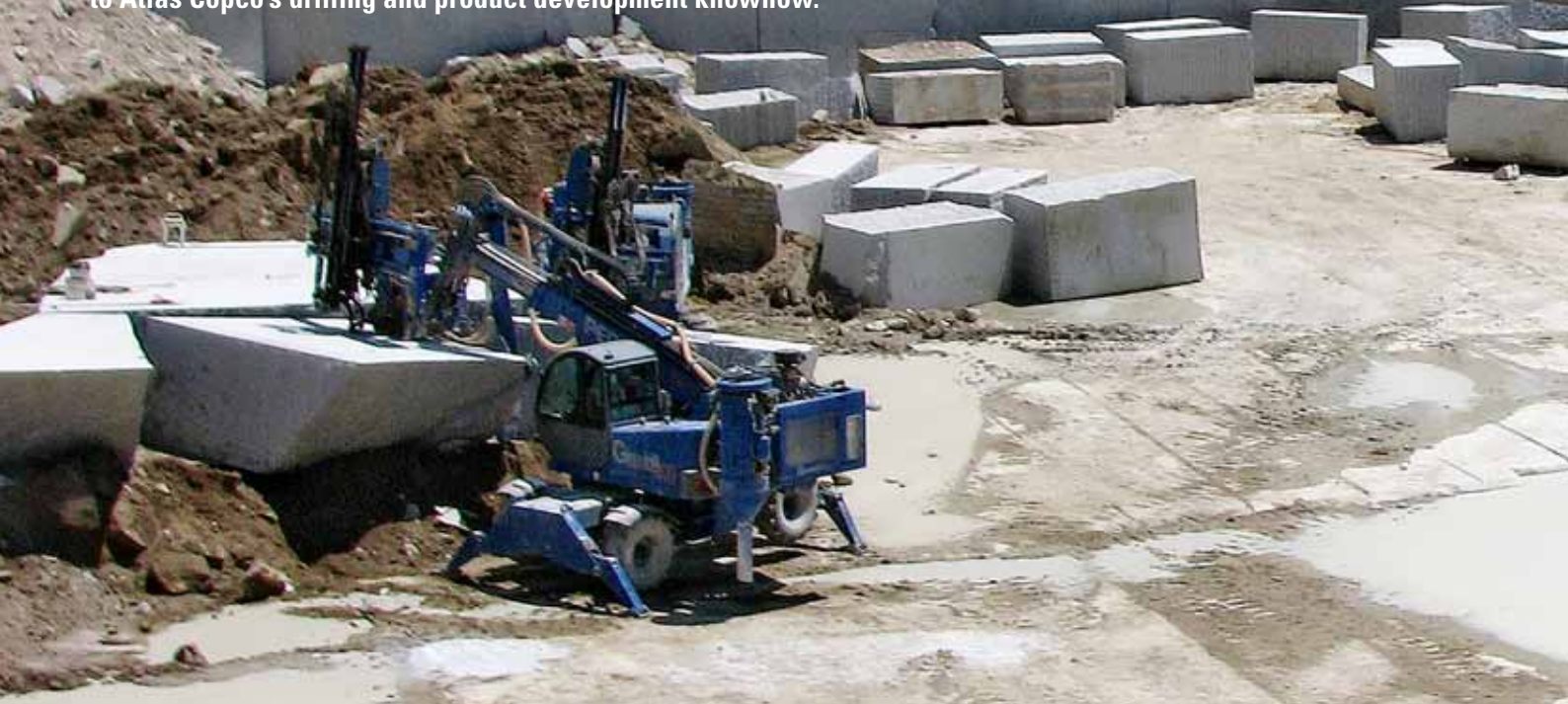
Perfora performance: Perfora's product range covers various types of hydraulic and pneumatic drill rigs as well as frames, hydraulic power packs, diamond wire saws and block splitting tools such as above at the Comita quarry in Sardinia and at the Augelli Marmi quarry in Puglia (insert).
