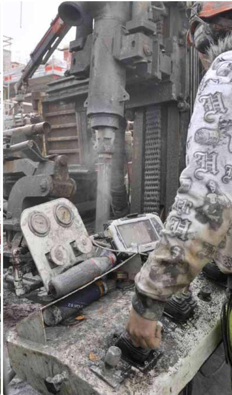
The perfect guide: The EDGE system feeds vital information to the operator, enabling him to continually adjust and optimize the process.
