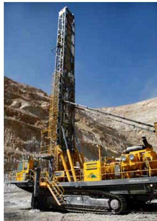
Best on site: The PV-351 has proved that it drills faster than the electric rigs in the Collahuasi fleet.
