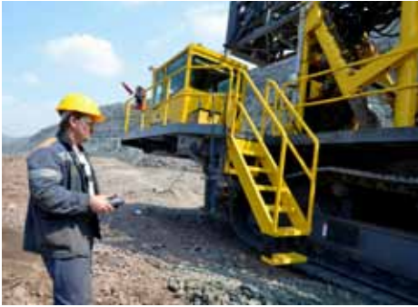
Drills of choice: The Pit Viper 275 is used at Poltava GOK to drill 251 mm blast holes for the production of iron ore pellets. These drills represent state-of-the-art large hole drilling technology.
