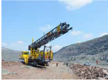
Drills of choice: The Pit Viper 275 is used at Poltava GOK to drill 251 mm blast holes for the production of iron ore pellets. These drills represent state-of-the-art large hole drilling technology.
