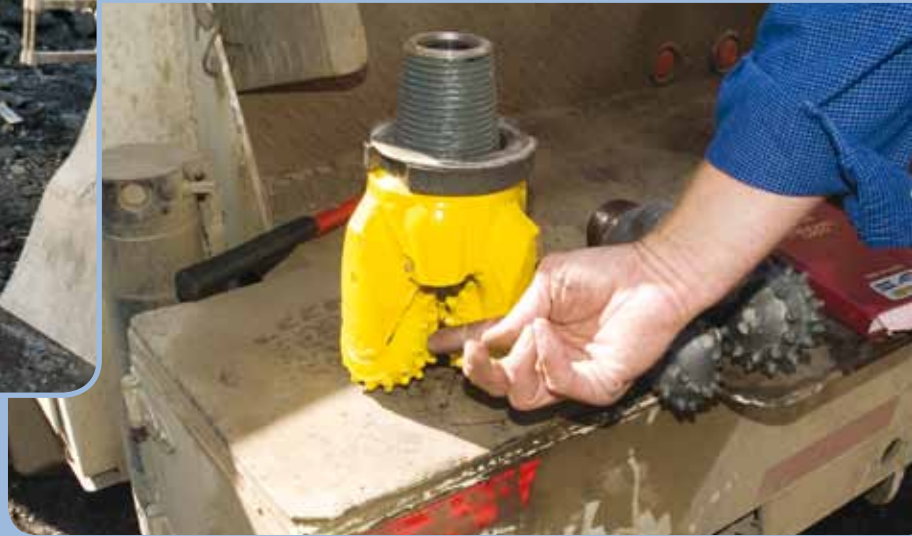
Drill mechanic Glenn Sharpe (left) is not changing bits as frequently. Mild steel pipe had been tougher on bit bearings.
