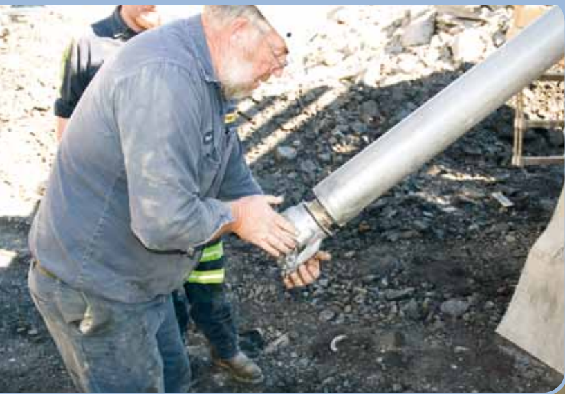
Drill mechanic Glenn Sharpe (left) is not changing bits as frequently. Mild steel pipe had been tougher on bit bearings.
