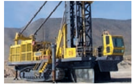
Bound for Kathu: The Pit Viper 351 which drills up to 406 mm (16") holes.
