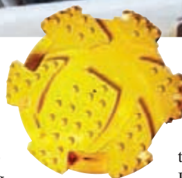
Good choice: The Elemex pilot bit that was attached to the inner drill string inside each casing.
