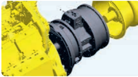
The patent pending automatic clutch system supplied as an option for selected rotary blasthole drill rigs. Right: A rig equipped with this system only uses compressed air for drilling and hole cleaning (yellow arrows).
