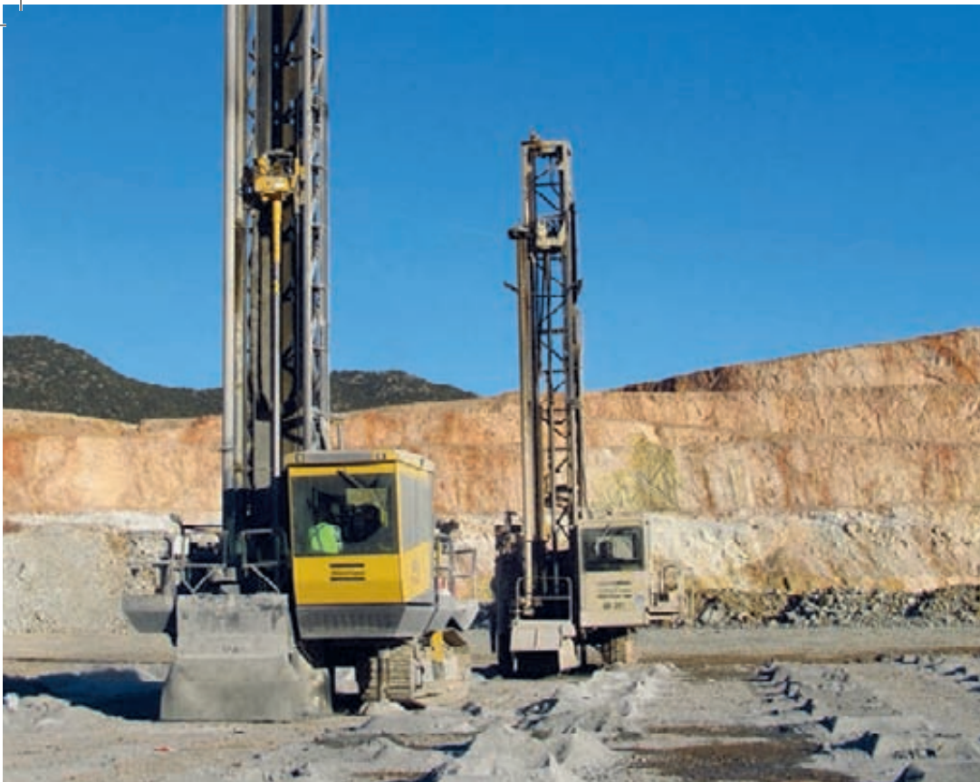
Good teamwork: The Pit Viper PV-235 above was delivered in mid-2011 and working together with two DM45 rigs, it helped to complete 650 000 drillmeters in 11 months.
