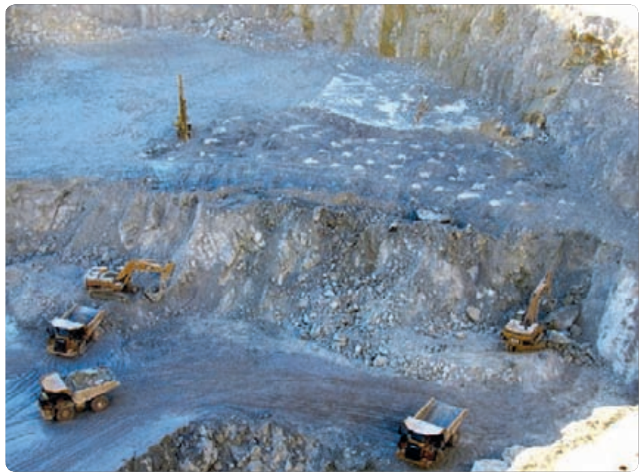
In full swing: Atlas Copco equipment is used in all phases of the operation in the Murgul pit, from drilling to haulage. Here, the benches are 10 m high and drilled with 2 m of sub-drilling with a pattern of 4 x 4 m in ore and 5 x 5 in waste.
