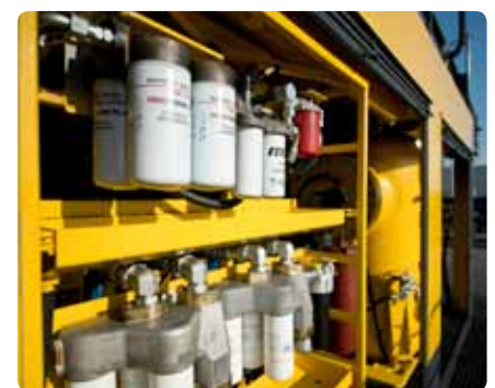
Easy service and maintenance: Above, the Pit Viper 311 rig's ground level access point and, below, the accessible filter rack.
