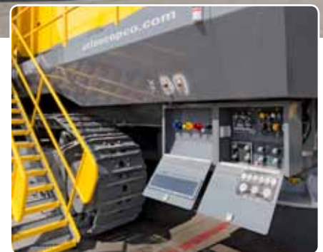
The PV-311, pictured above before its debut at MINEexpo 2012, is standard equipped with RCS Basic. This allows customers to start at a low level of automation and later add new functionality as their requirements change. RCS also provides the rig with a number of safety interlocks, protecting both the operators and the equipment.
