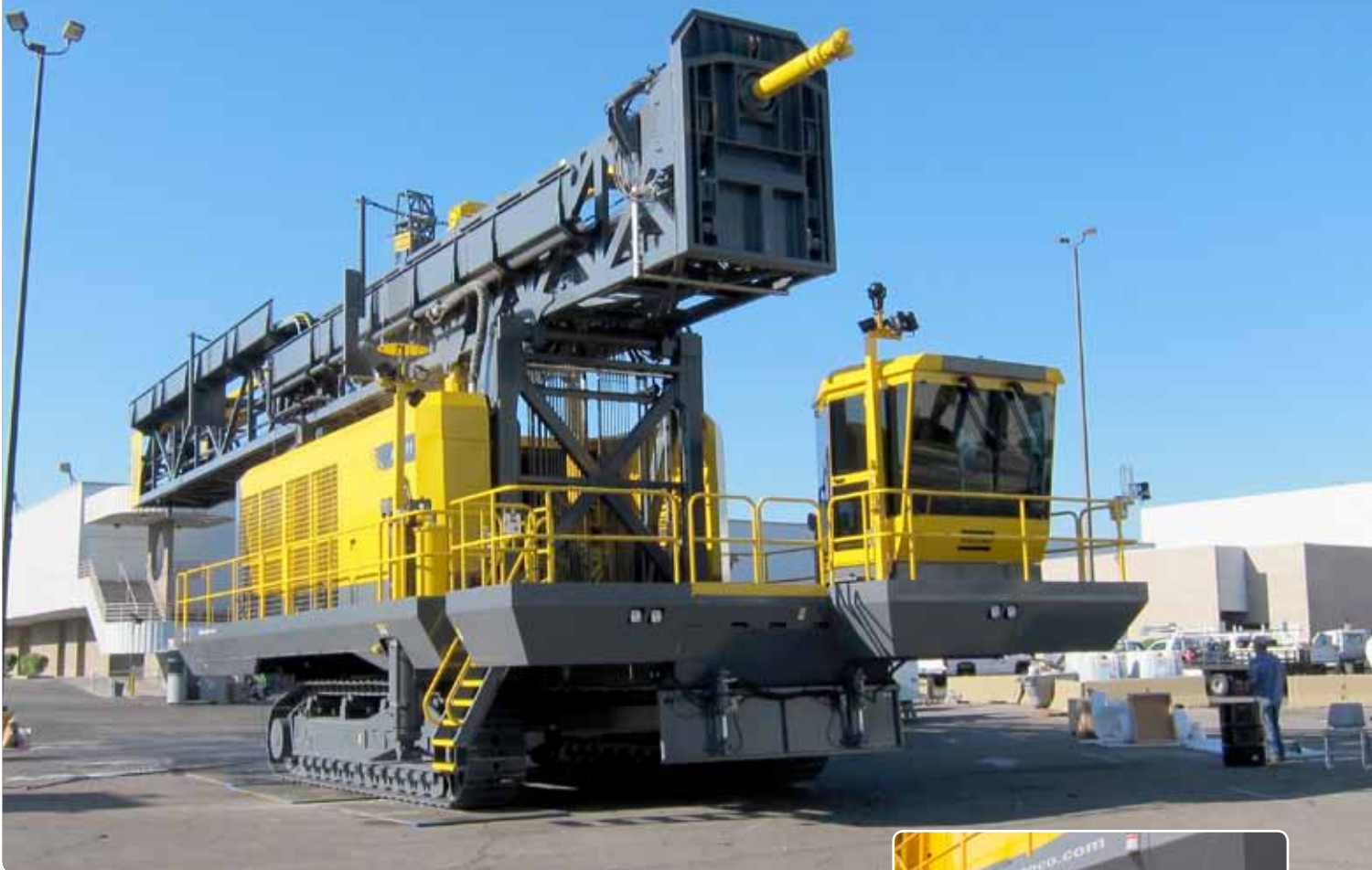
The PV-311, pictured above before its debut at MINEexpo 2012, is standard equipped with RCS Basic. This allows customers to start at a low level of automation and later add new functionality as their requirements change. RCS also provides the rig with a number of safety interlocks, protecting both the operators and the equipment.
