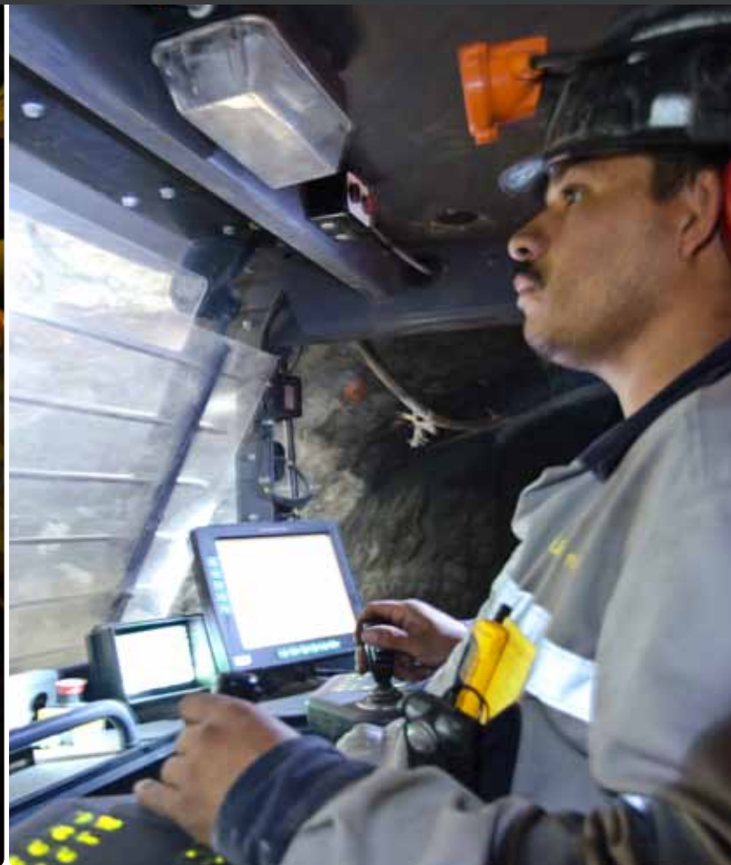
In control: During M&C's visit, a Scaletec operator demonstrated how the rig is used to scale the walls in the drifts and remove loose rock in new stopes.
