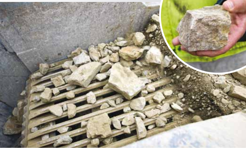
For many of Schotterwerk Moersdorf's customers, consistent cubic fractions are a necessity, since their geometry provides superior compaction.
