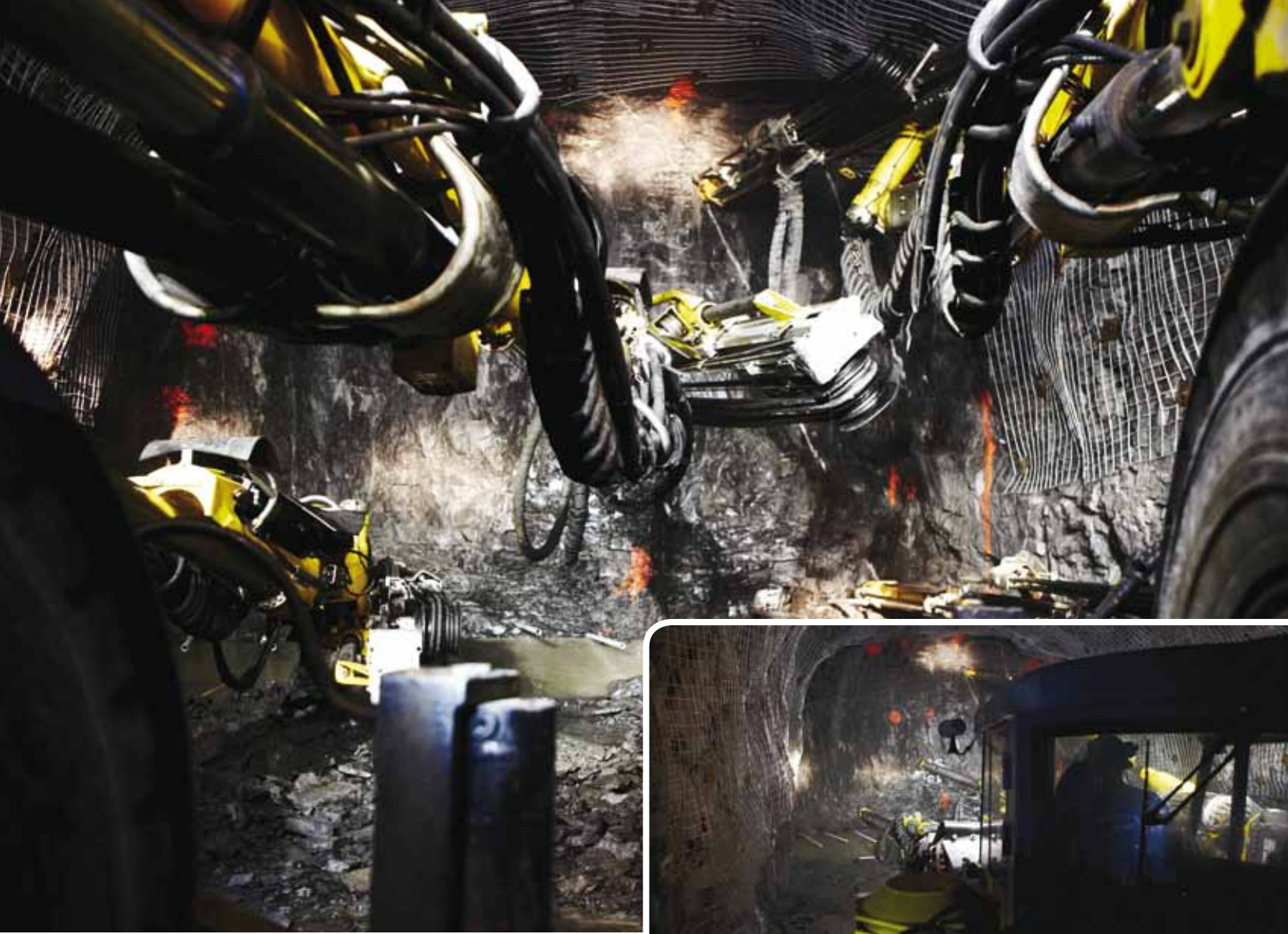
(above) The drills have been operating well and two new Boomer M2 C rigs will join the two already at Project Eleonore later this year. Photos courtesy The Redpath Group
