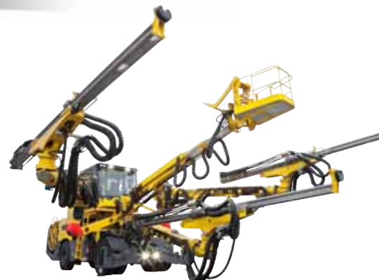
Boomer XE3 C: Computerized and unbeatable for driving road and rail tunnels. At Bauma it will feature the new COP 4038 rock drill.
