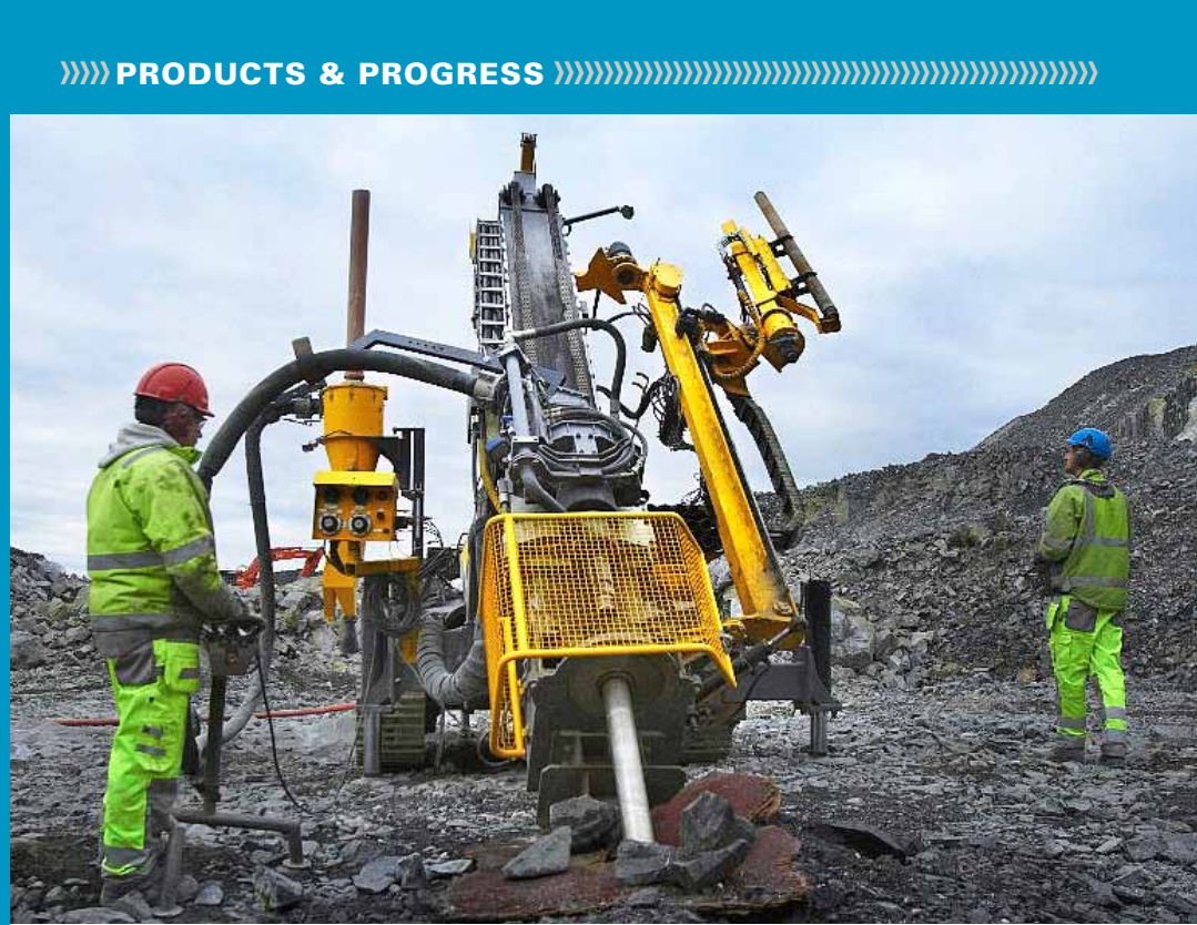
Committed to RC drilling: the new Explorac 100 is compact yet powerful, featuring an automated rod handling system and benefits for personal safety in the field.
