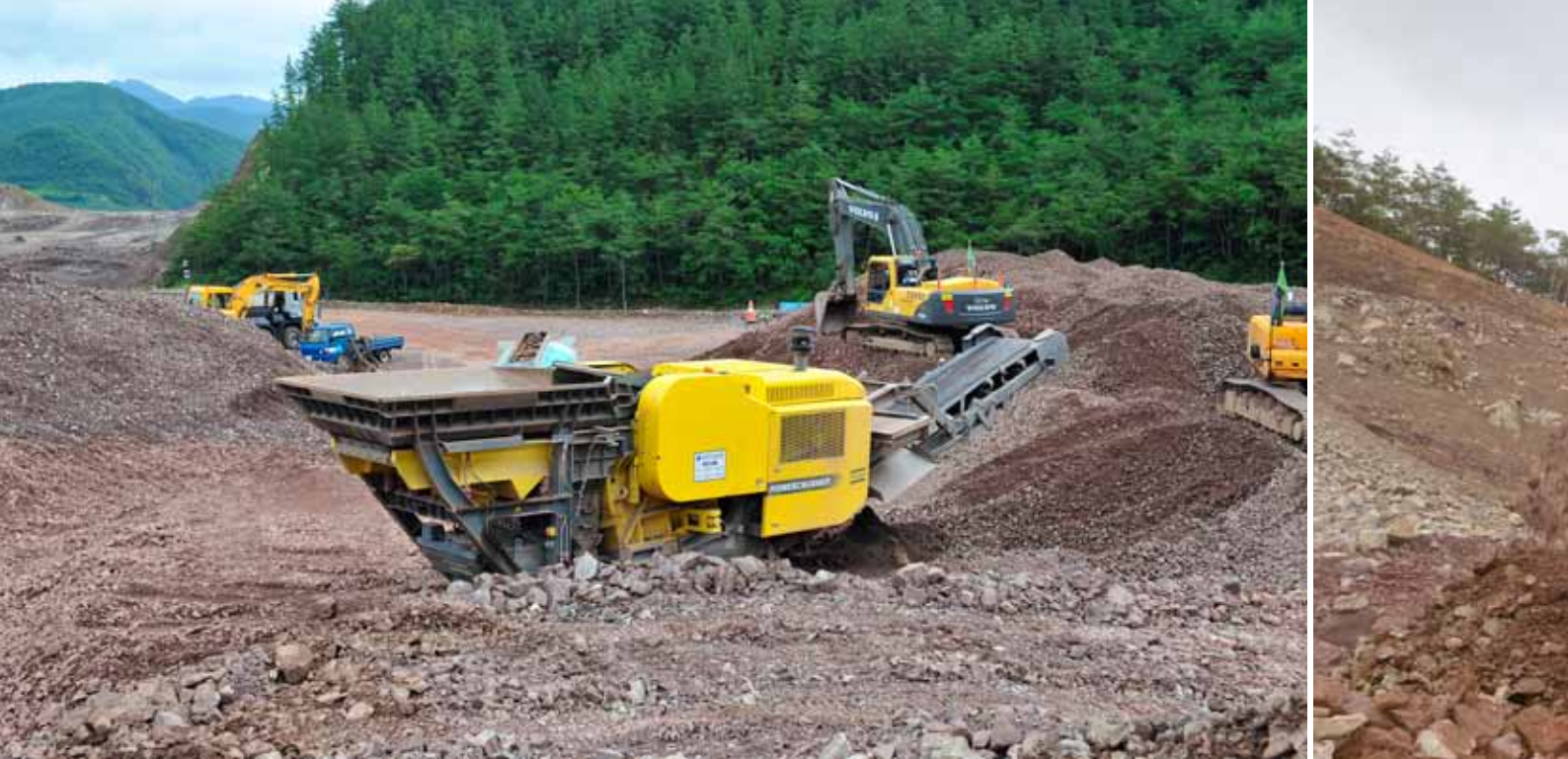
Quarrying for the future: Wonjin Construction puts the Powercrusher PC 4 to work to supply aggregate for Korean infrastructure expansion, pictured at a site in Andong along the construction route of the new Highway 30.
