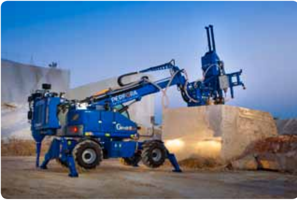
Carefully selected: The Girodrill EVO drills a marble block at the Pinoso quarry in Alguena. Above, Quarry Manager Jesús Pérez de la Muela (right) with Fernando Menendez, Atlas Copco's Business Line Manager in Spain.
