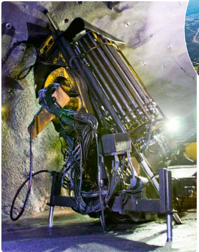
Above, operator Andreas Larsson during one of the few occasions he goes into the drift to reposition the rig for the next fan of blastholes. Right, the Simba WL6 C in full fan drilling mode, drilling 30 m long holes at the center of the fan and 17 m holes on the sides.
