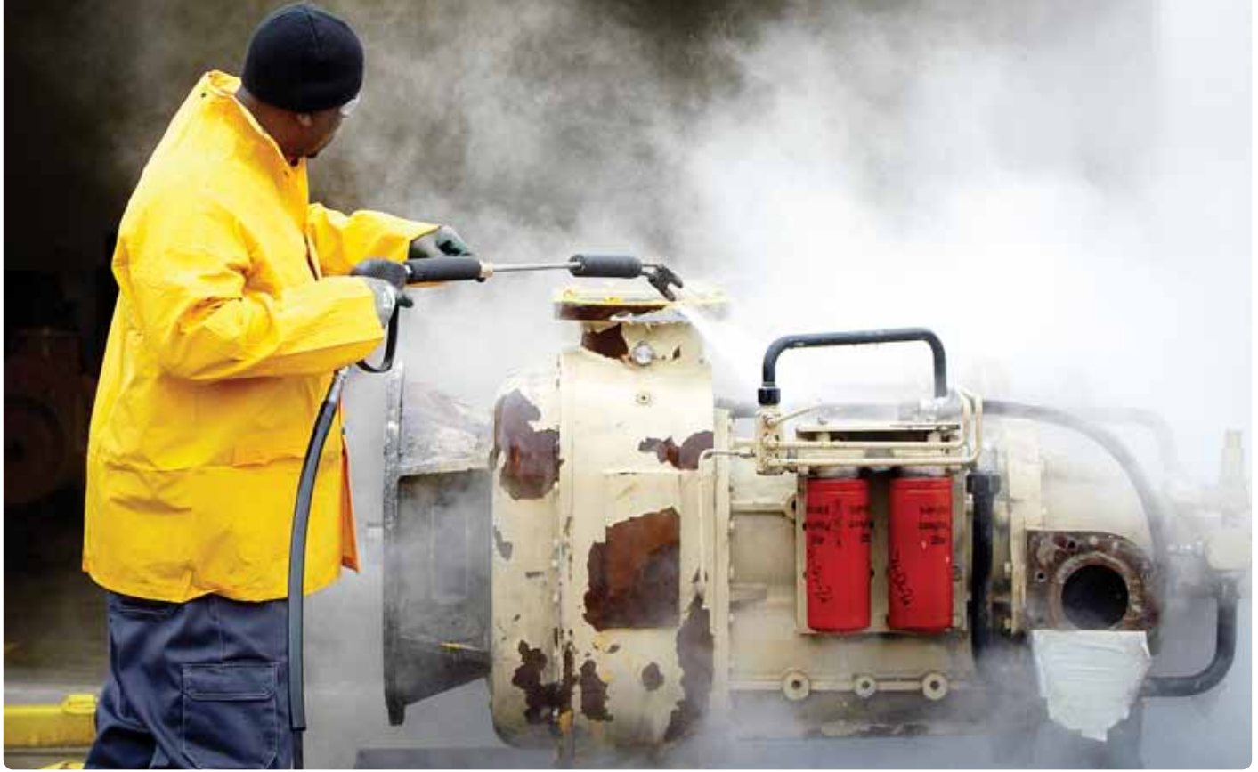
Remanufacturing in the USA: The process begins with the cleaning of all components before moving on through the five remanufacturing work bays. The procedures and processes developed in Garland set the standard for Atlas Copco Reman Centers worldwide.
