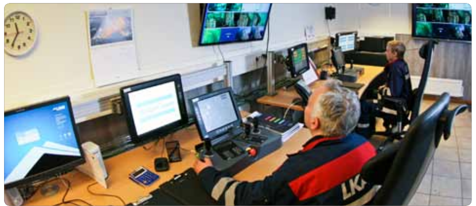
At a safe distance: The Malmberget control room where each operator is in charge of two Simba drill rigs. Here, Production Supervisor Bengt Anttila checks data logs from the night's drilling.
