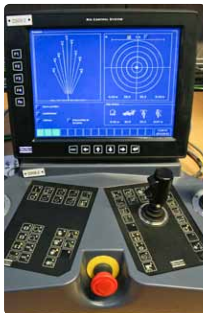
Teleremote technology: Above left, the drill plans for the Simba WL6 C rigs as they appear on the operator console. Right, the screen setup that monitors the progress of each rig in the mine.
