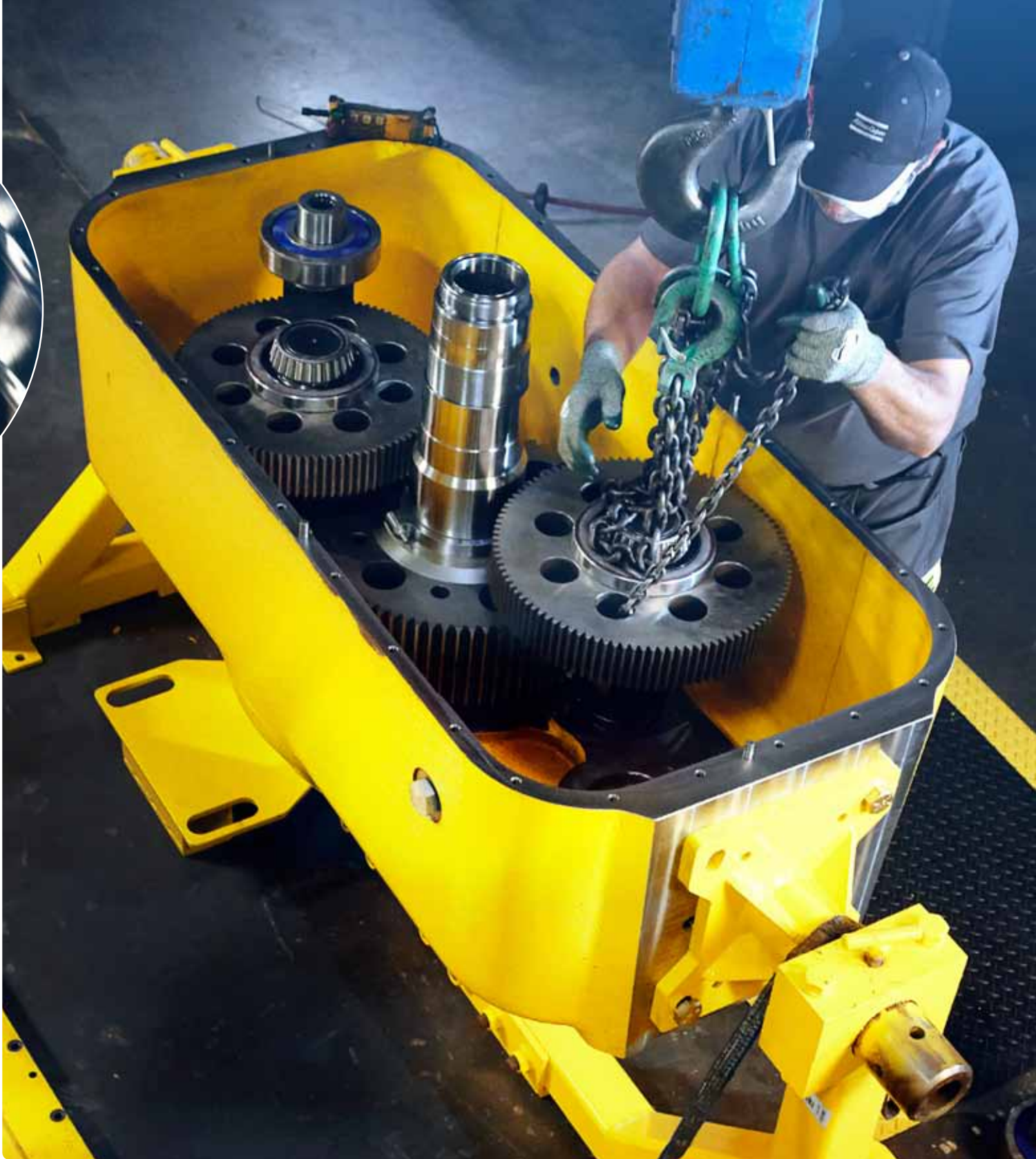
Remanufacturing in action: This rotary head from a Pit Viper 351 drill rig will be completely restored and reassembled using new genuine parts and applying the latest engineering specifications and factory upgrades.
