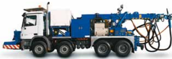
Roadrunner: Sprays wet concrete and the only MEYCO unit which can be transported on ordinary roads.
