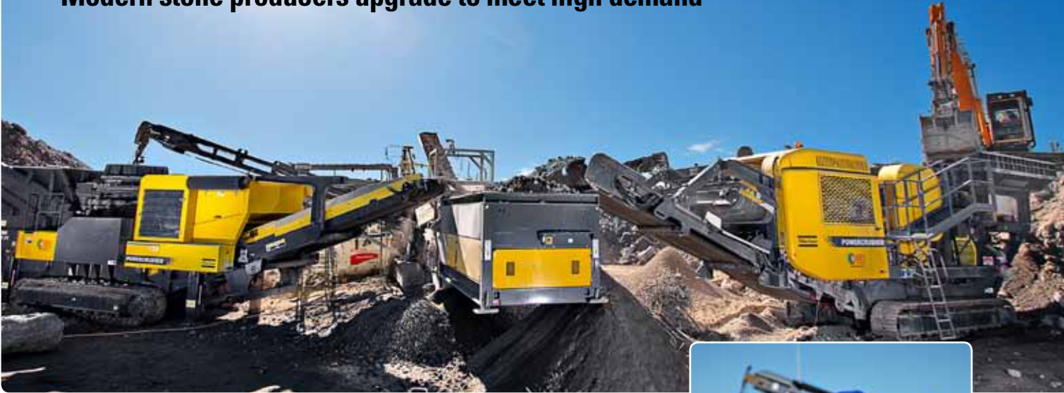
Fleet of power: At the Boral recycling site at Kooragang Island, MES has installed both a Powercrusher PC 6 and PC 21 mobile crushing unit as well as an HCS 5515 screening unit.
