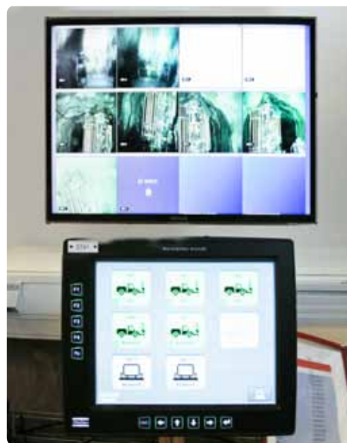
Teleremote technology: Above left, the drill plans for the Simba WL6 C rigs as they appear on the operator console. Right, the screen setup that monitors the progress of each rig in the mine.
