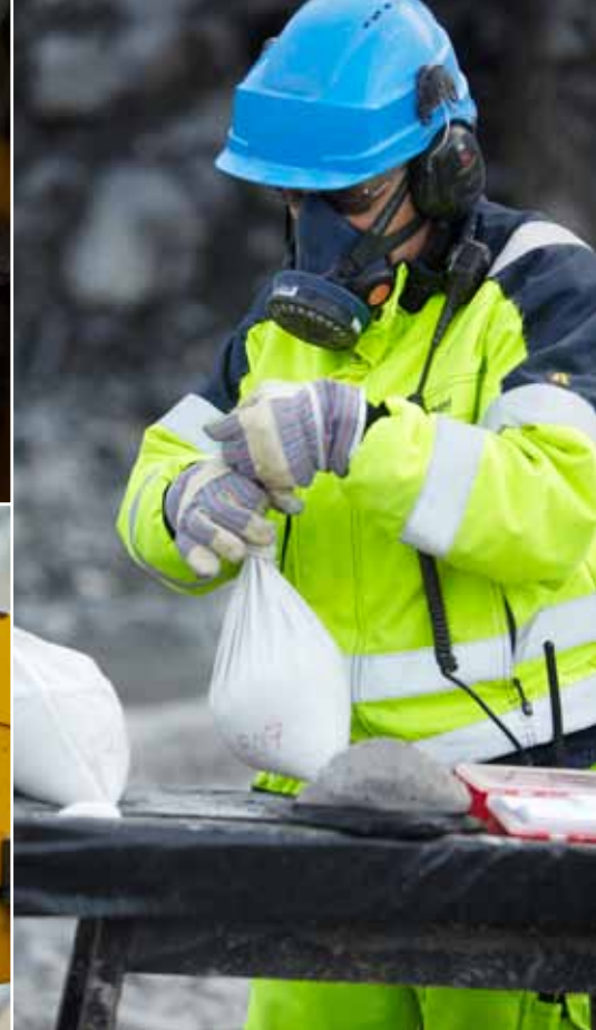
The art of grade control: Identical sample fines weighing 2.5 kg are a prerequisite for accurate analysis.
