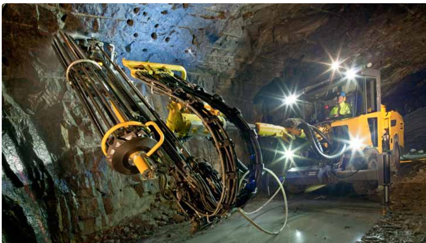
The new Boltec S for small tunnels and drifts: It can be used for the safe installation of bolts from 1.5 to 2.4 m in length.
