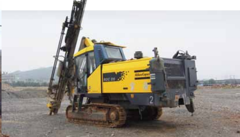
... drilling for limestone aggregates with the FlexiROC T40...
