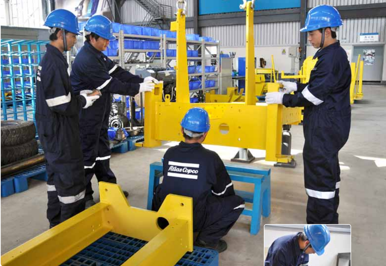
Technicians at the Kunming Reman Center assembling the main frame of a Boomer 281 drill rig.
