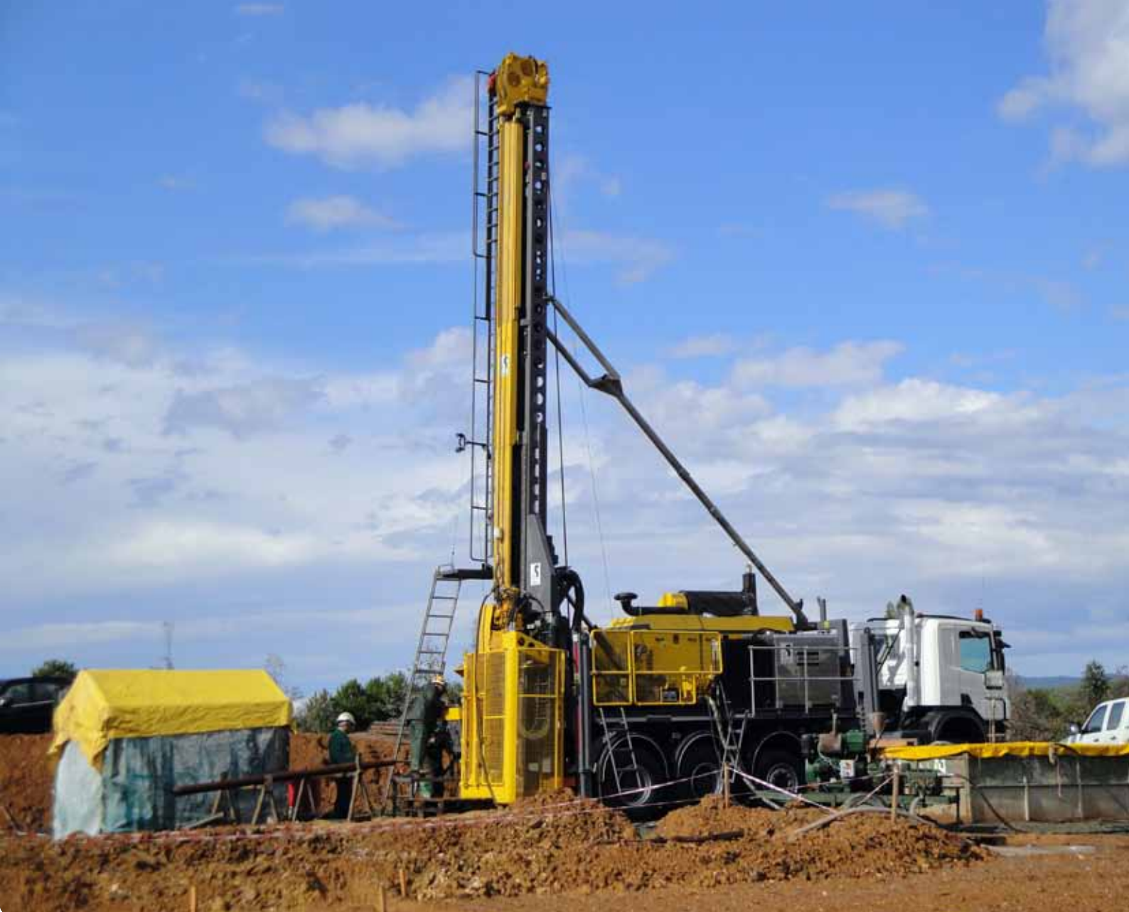
The Atlas Copco exploration rig Christensen CT20: Initially, the rig did not perform to the best of its ability at the Rio Tinto mine in southern Spain, but after changing the drilling parameters and with extra training for the crew, the results exceeded expectations.
