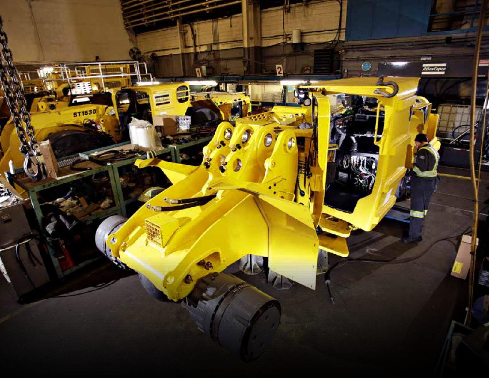
A team of reman specialists bring the ST 1520 back to the exact specifications of the original. Atlas Copco stands behind the rig, giving it a new rig warranty and presenting the customer with complete documentation of every step of its reman process.
