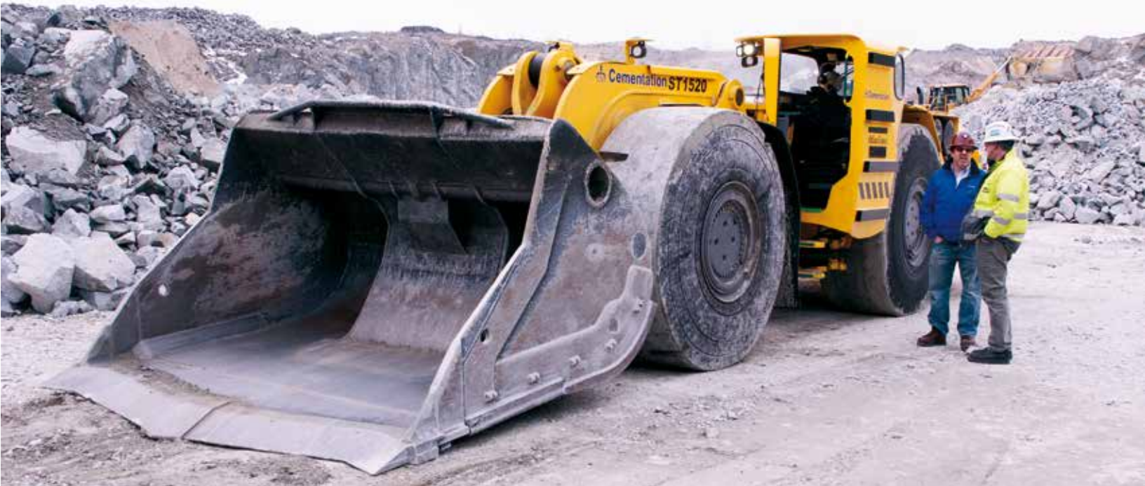
Above, Cementation Equipment Manager Ernie Schaffernicht (left) and Atlas Copco salesman Aaron Walsh discuss the rebuilt Scooptram ST1520 as it goes through final tests.
