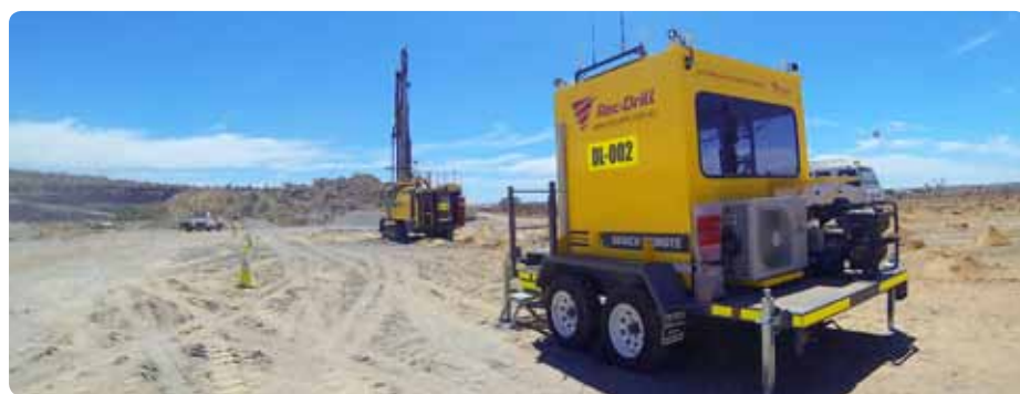
Available from mid-2014: The BenchREMOTE station allows the surface drill rig operator at a potentially hazardous worksite to control the rig from a safe distance of up to 100 m.
