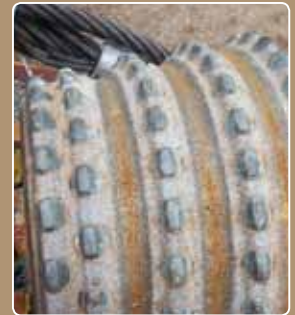
High quality and long life: Left, Magnum cutter G and Magnum cutter N (right) after reaming the 307 m shaft.
