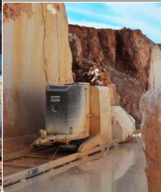
Below: The machine is easy to set up and the tracks can be lifted together with the machine.
