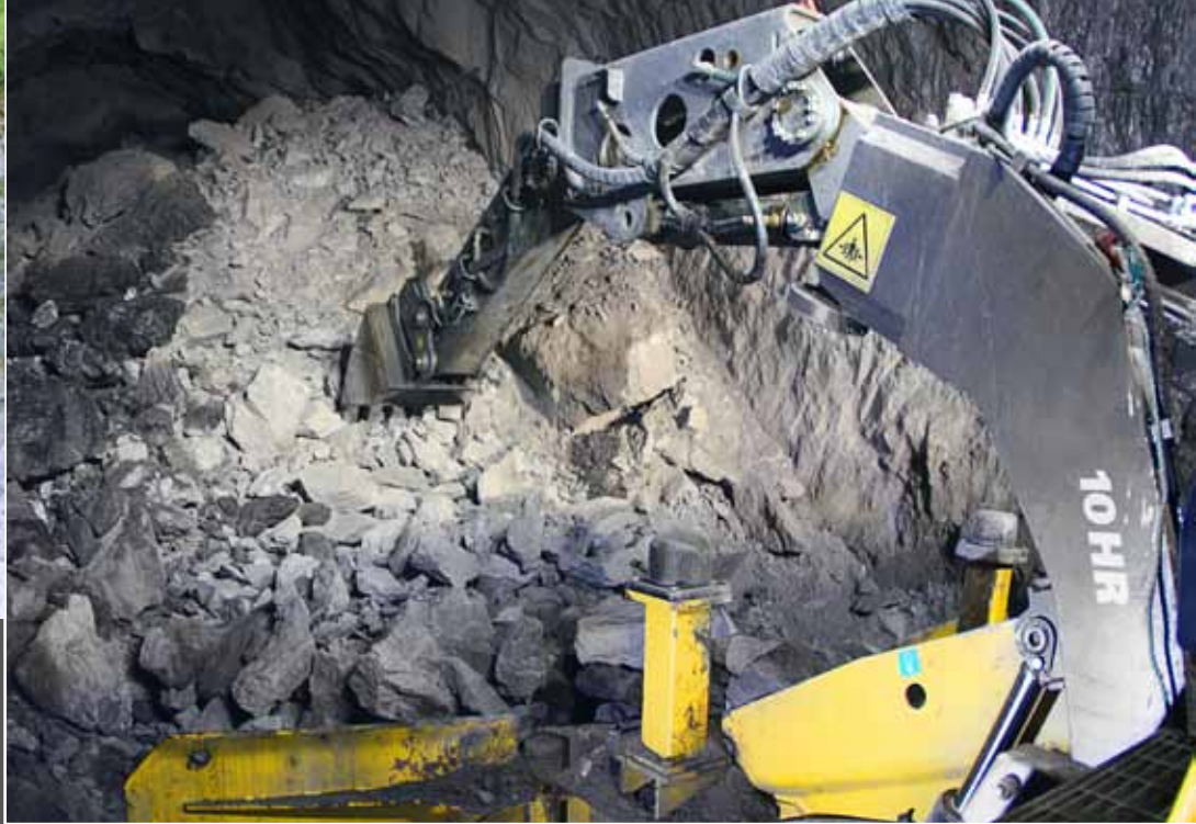
The Häggloader's backhoe digger shovels blasted rock from the muckpile onto the conveyor. Below, the conveyor dumps the muck straight into the waiting truck.
