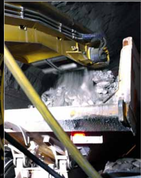
The Häggloader's backhoe digger shovels blasted rock from the muckpile onto the conveyor. Below, the conveyor dumps the muck straight into the waiting truck.
