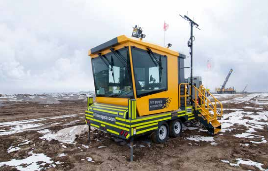
This mobile remote Pit Viper operator station is a purpose-built solution to teleremotely control a Pit Viper from outside the pit. Video cameras send the driller a live feed as though he were on the rig. Distance is limited only by the capabilities of the communication network used for transmission. Customers have the option to use their own network or a radio network set up by Atlas Copco dedicated to teleremote operations.
