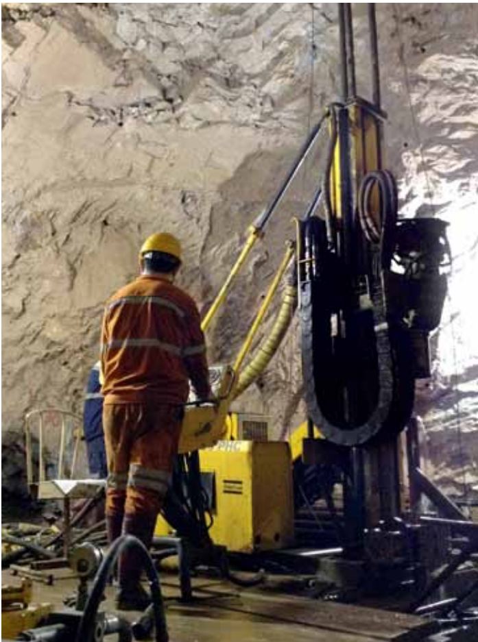
Record-breaker number one: The Diamec U4 in its 5 x 6 m drift.
