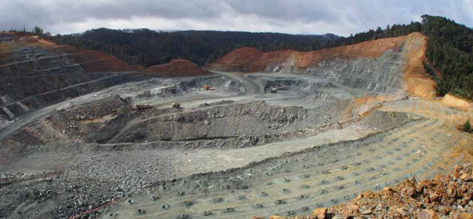
View of the Savage River mine: Heavy rainfall in the area can sometimes affect the stability of the benches. Atlas Copco's BenchREMOTE system enables the SmartROC D65 drill rig to be operated from a safe distance.
