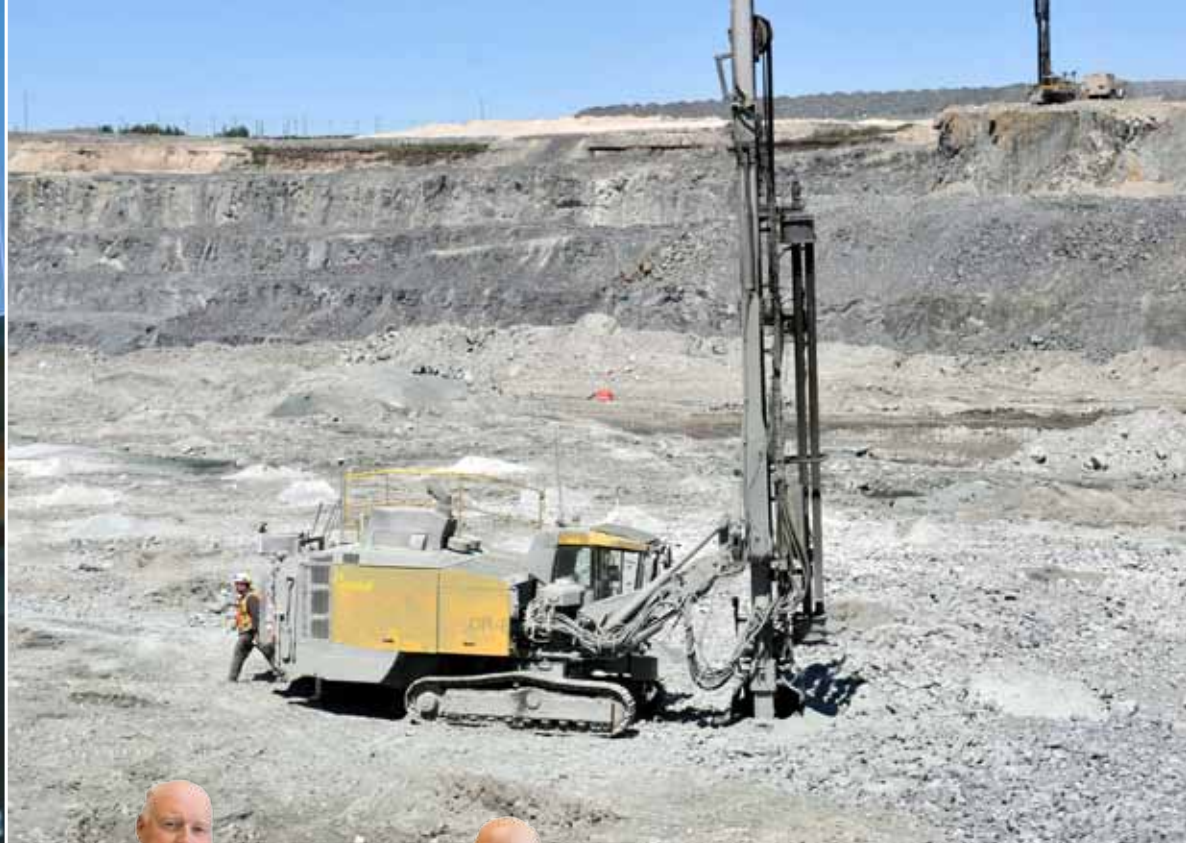
Good combination: A SmartROC D65 (foreground) with the Pit Viper 271 in the distance (top right).
