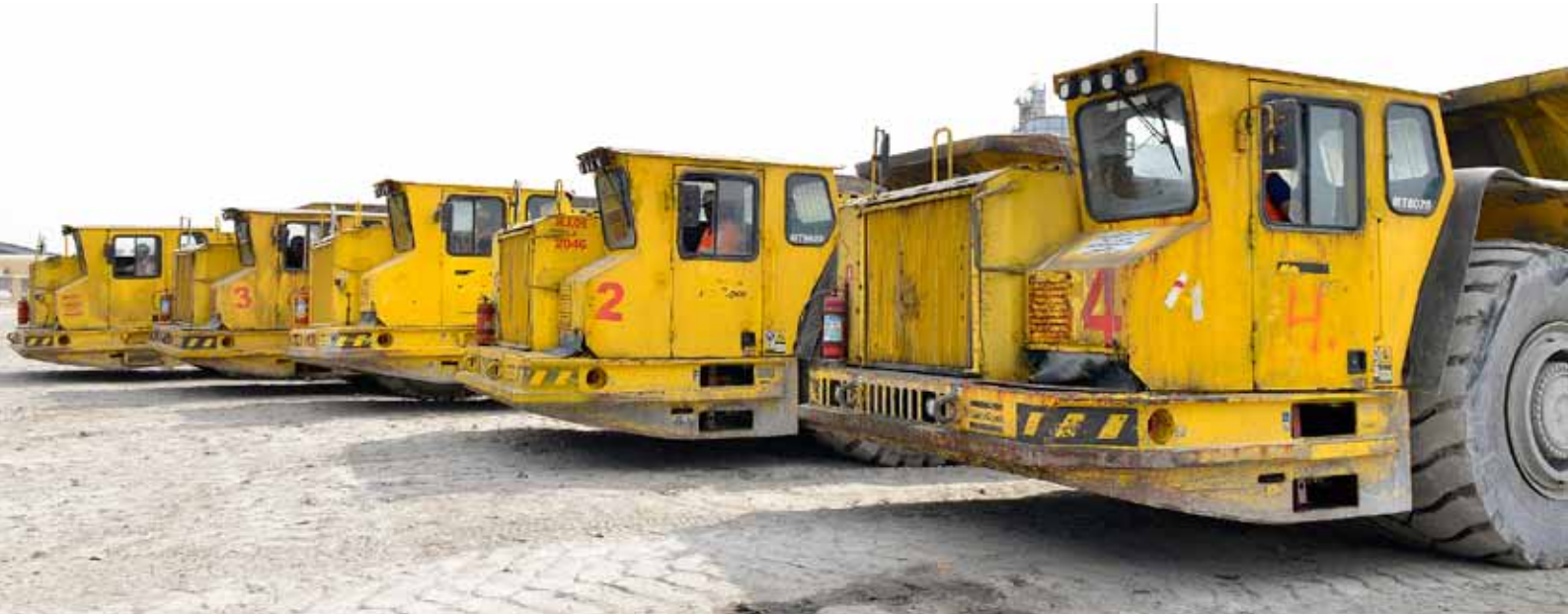
Impressive lineup: Part of HZL's large fleet of Atlas Copco mine trucks at Rampura Agucha, mainly consisting of the 60-tonne Minetruck MT6020.
