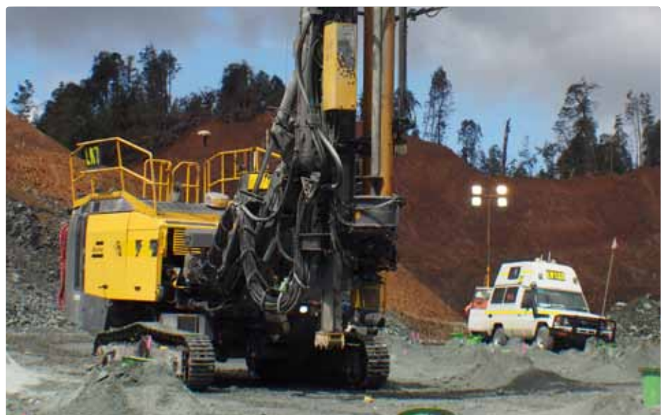
When bench stability is in doubt: The Atlas Copco SmartROC D65, seen here together with the BenchREMOTE unit mounted inside a vehicle (right) at the Savage River Mine in Tasmania.
