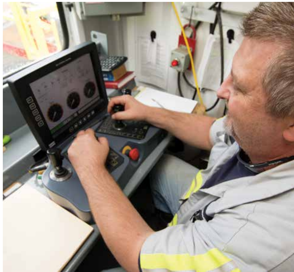
▲ Raisebor's James Bass operates the 123RH C raiseboring machine from the quiet comfort of its remote operator station.
