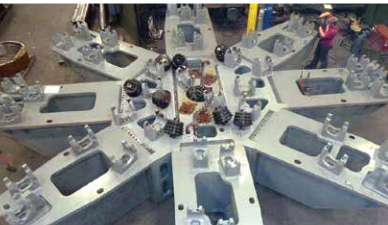
▲ Atlas Copco Secoroc cutters for the raise bore reamer.
