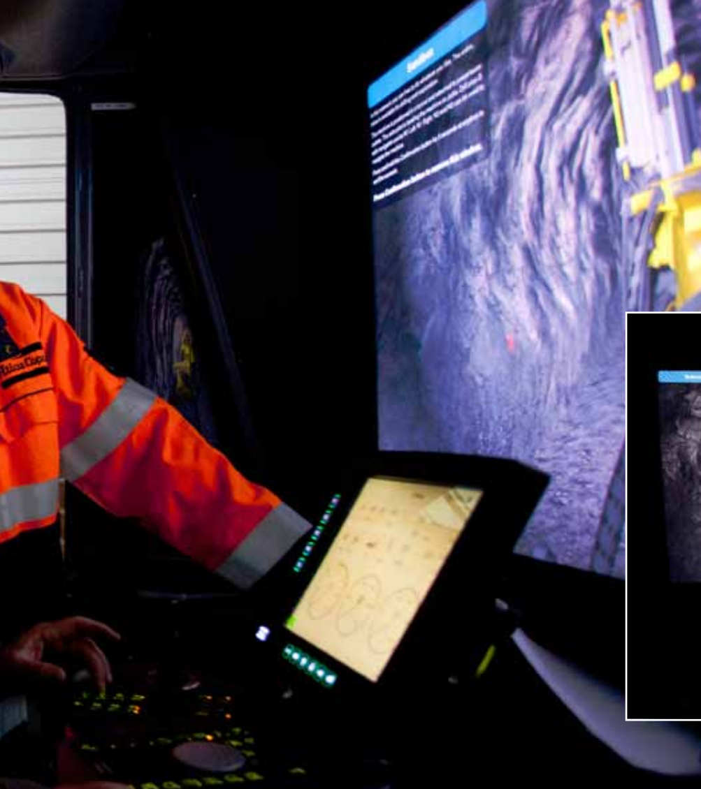
Personal trainer: Trainees are instructed at every level on how to perform drilling procedures in the simulator with no impact on the mine's actual operations.
