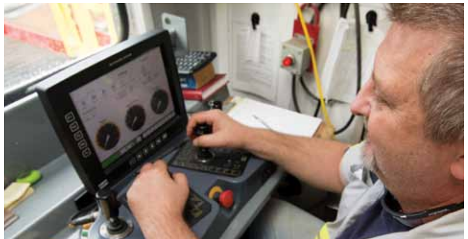
Raisebor's James Bass operates the Robbins 123RH C raiseboring machine from the quiet comfort of its remote operator station.
