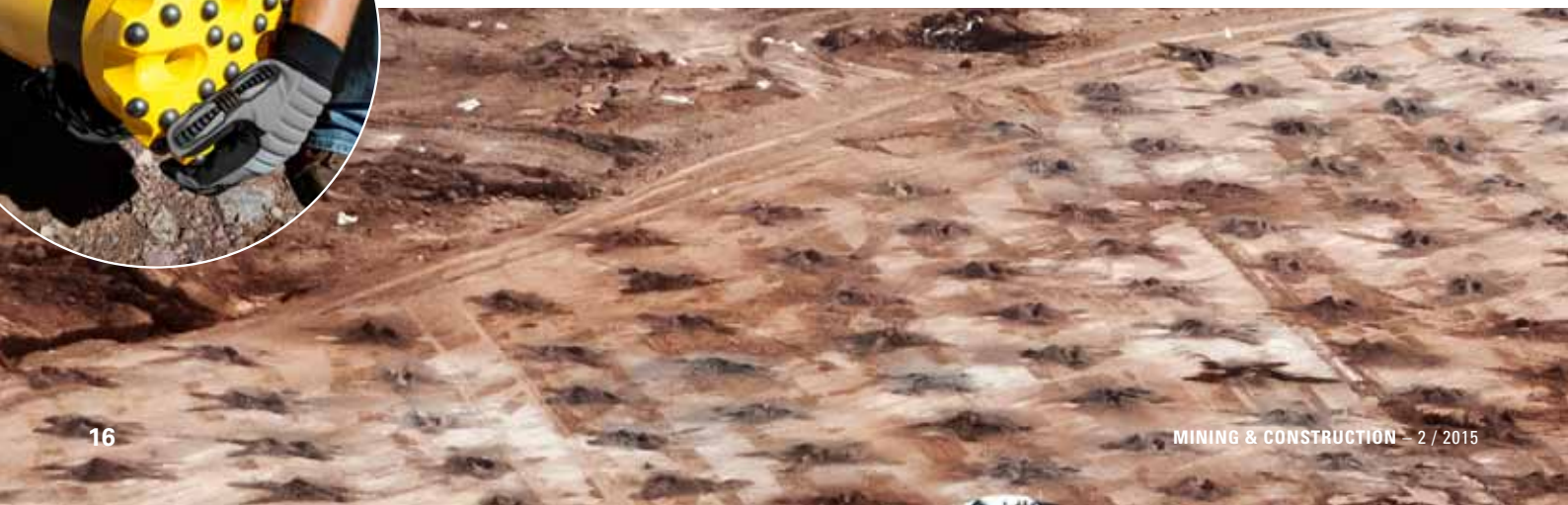
The Secoroc COP 86 weighs 201 kg (443 lbs) which is lighter than previous models making it easier and safer to handle.
