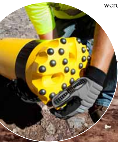
The Secoroc COP 86 weighs 201 kg (443 lbs) which is lighter than previous models making it easier and safer to handle.
