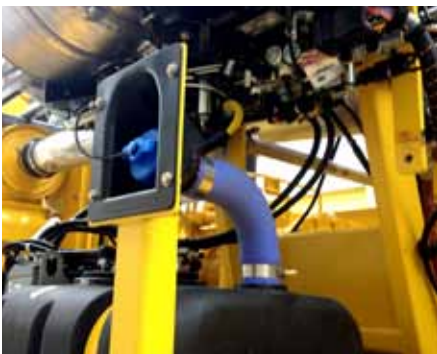
The easily recognizable blue refill cap and hose on the Pit Viper.
