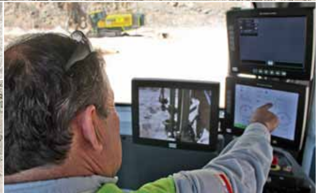
Times are changing: Left, the SmartROC D65 drills by itself while the operator (right) controls all functions from a safe distance.
