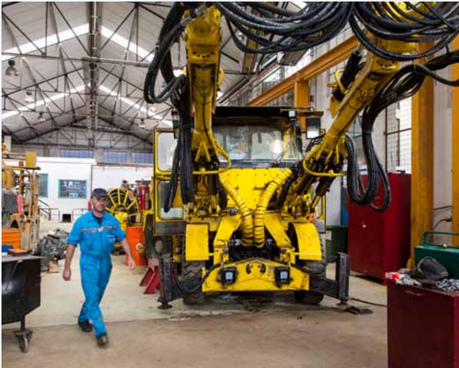
Part of the fleet: The Atlas Copco Boomer 128, used in the construction of access roadways from the main ramp, during service and maintenance in the Aljustrel workshop.
