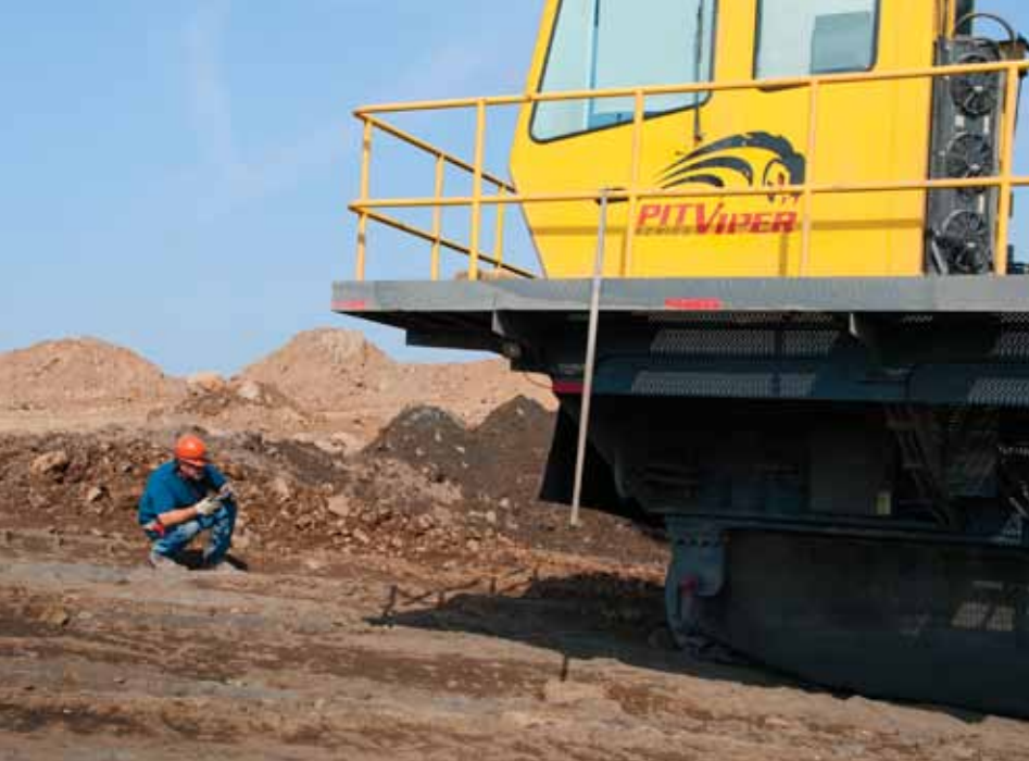
The perfect complement: Unlike electric drill rigs, the diesel-powered Atlas Copco Pit Viper 351 provides Minntac Mine with a high level of mobility. This enables the rig to be moved easily and quickly to any part of the pit.
