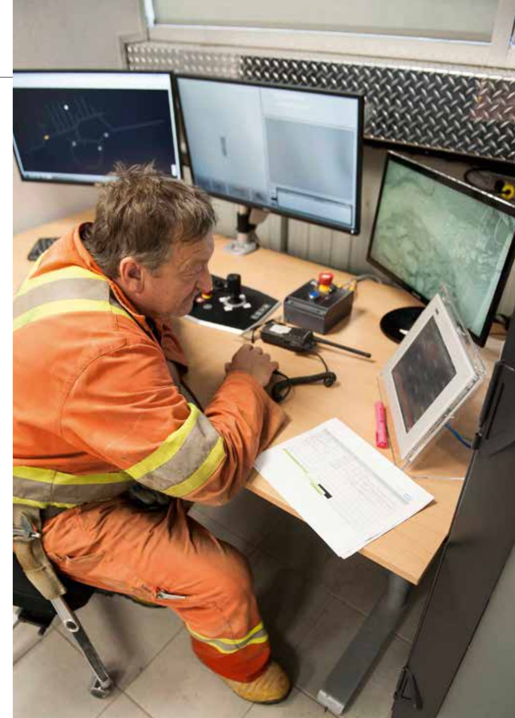
Operator Wayne Locht switches the Scooptram ST14 to remote control mode in the automation zone 1.4 kilometers below.
