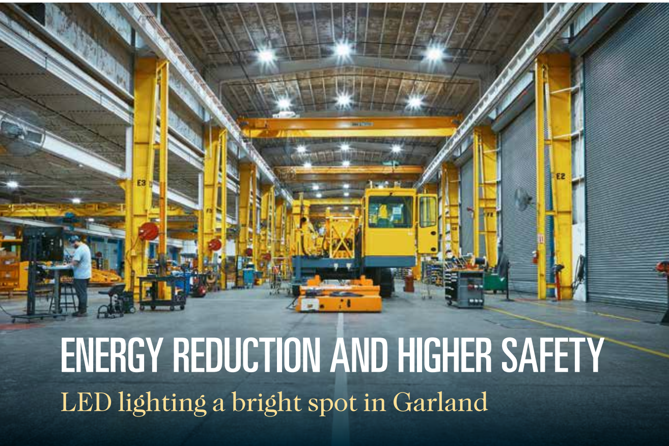
← Energy consumption at Epiroc's Garland production facility has gone down from about 1.3 million kilowatt hours to roughly 397 000, thanks to LED lights.
