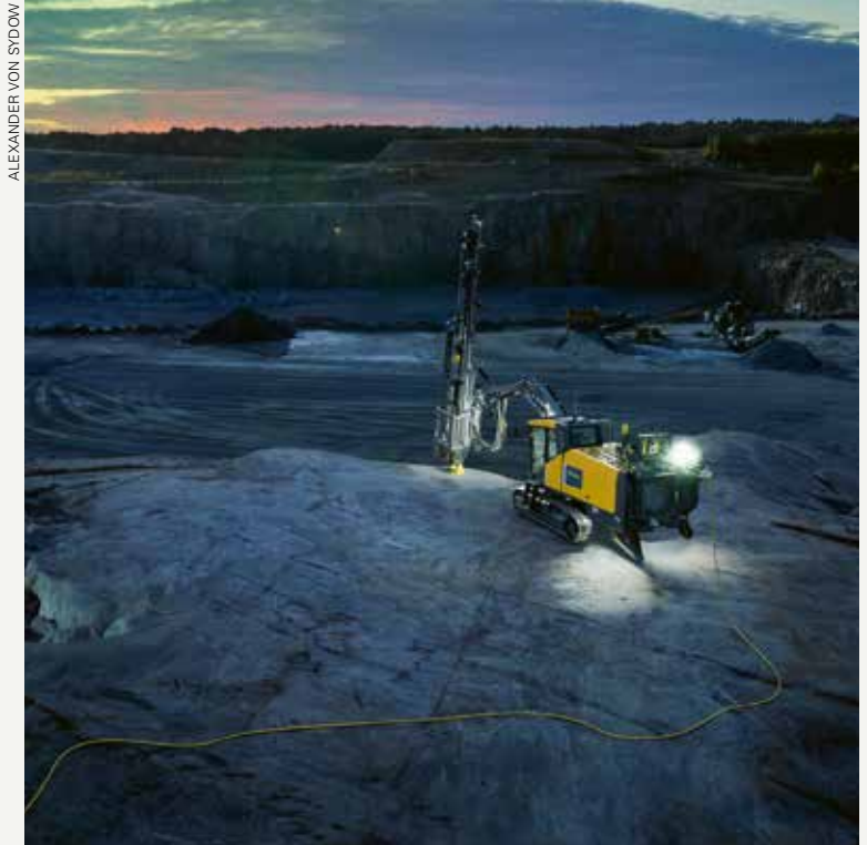
The SmartROC T35 E is being trialled by Skanska in the Stockholm area. The rig is an important step in the shift toward zero-emission drilling in surface mines and quarries all over the world.
