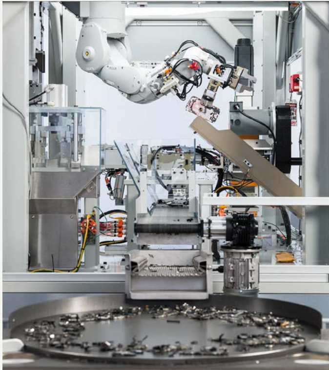
Daisy, less than 20 yards in length, uses a four-step process to remove an iPhone battery with a blast of -80 degree Celsius air, and then pop out screws and modules.
